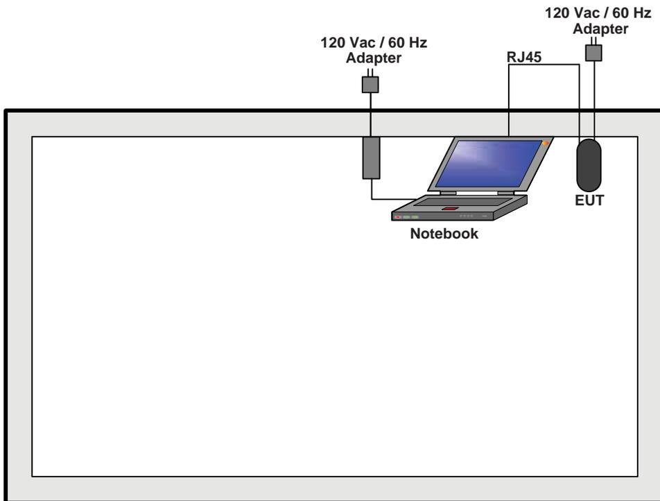
For radiated emissions 9kHz~1GHz
