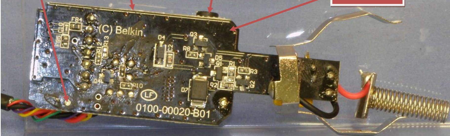
Photo 10 - Bottom Side of Transmitter/Power Board
