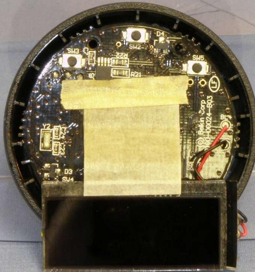
Photo 11 – Top side of Processor Board
