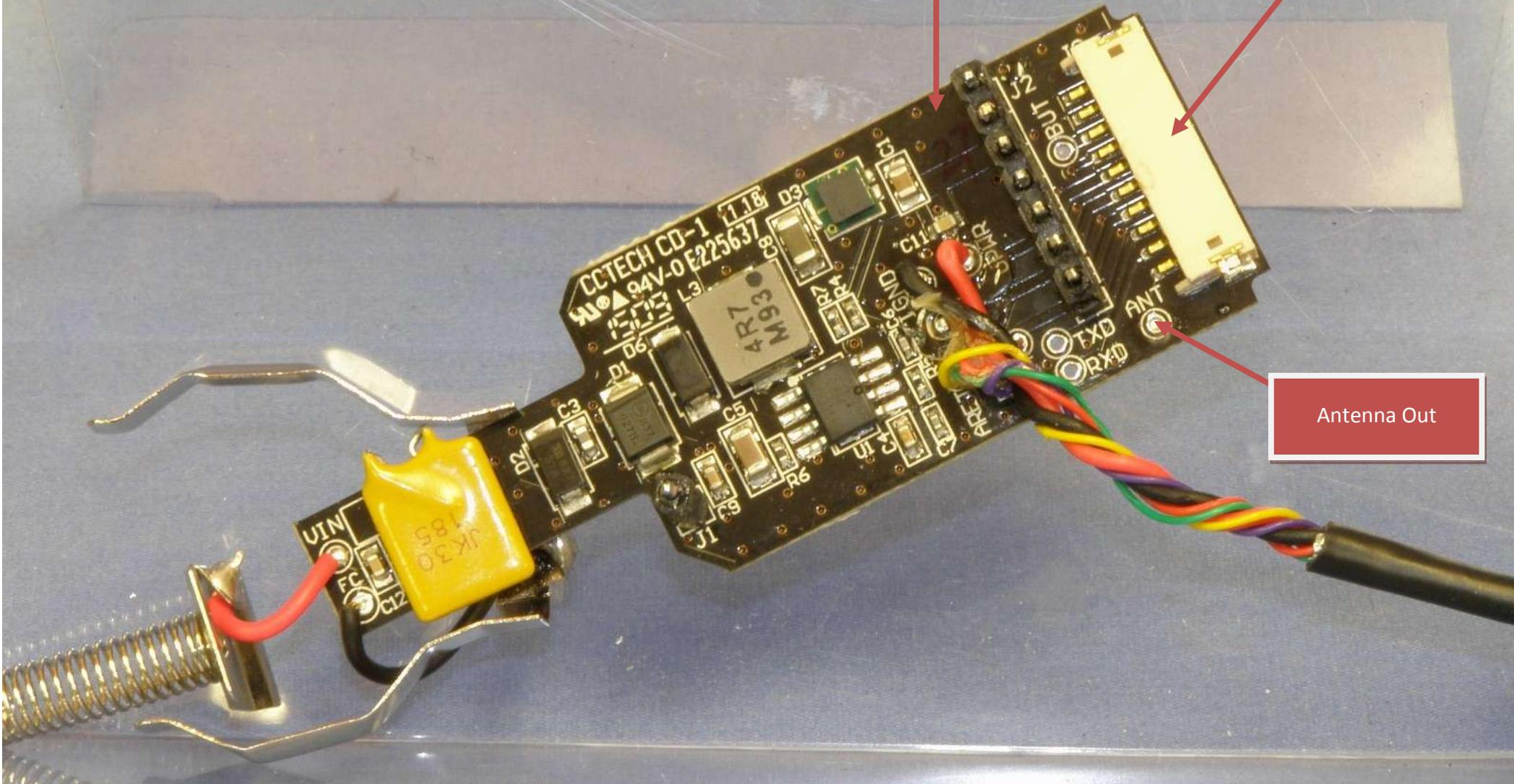
Photo 9 - Top Side of Transmitter/Power Board
