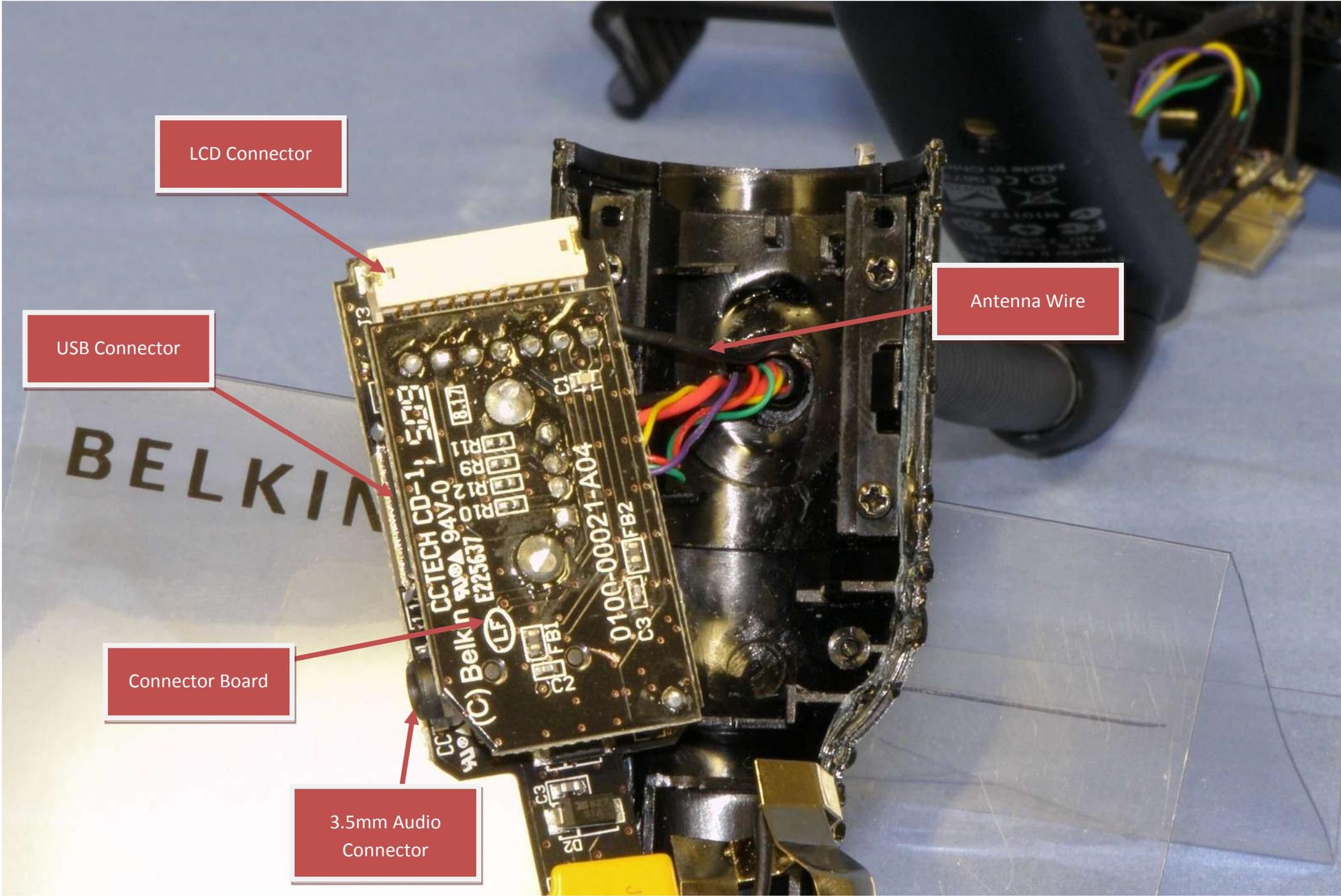
Photo 7 - Top Side of Connector Board
