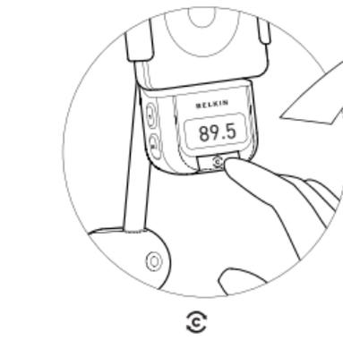
**3. CLEARSCAN (Automatic frequency selection)** Press "ClearScan". TuneBase FM displays the best frequency.
