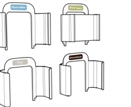
**2. Select correct cradle for your iPod.** Cradles are marked in front with compatible iPod.
