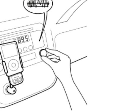
**7. Match station using up and down buttons.**
