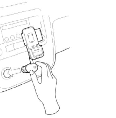
**1. Remove iPod and insert TuneBase FM into power outlet.**
