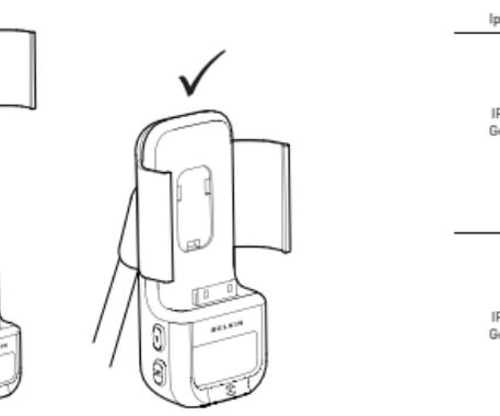
**3. Slide cradle into open slot in TuneBase FM until it latches in. Test-fit your iPod.**
