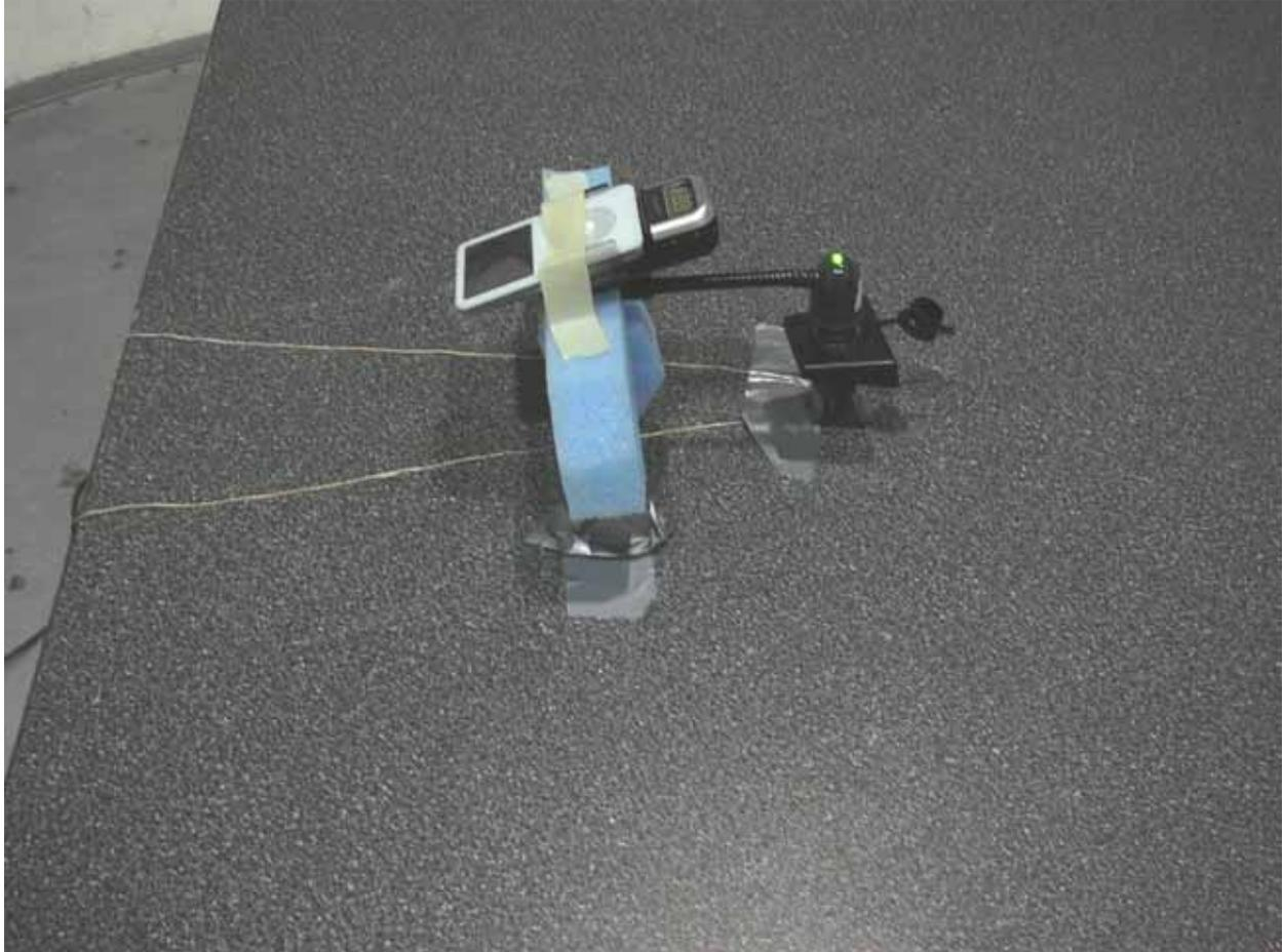
Test Setup: 9 kHz to 30MHz Radiated Emission at 3 Meter Distance – Facing EUT
