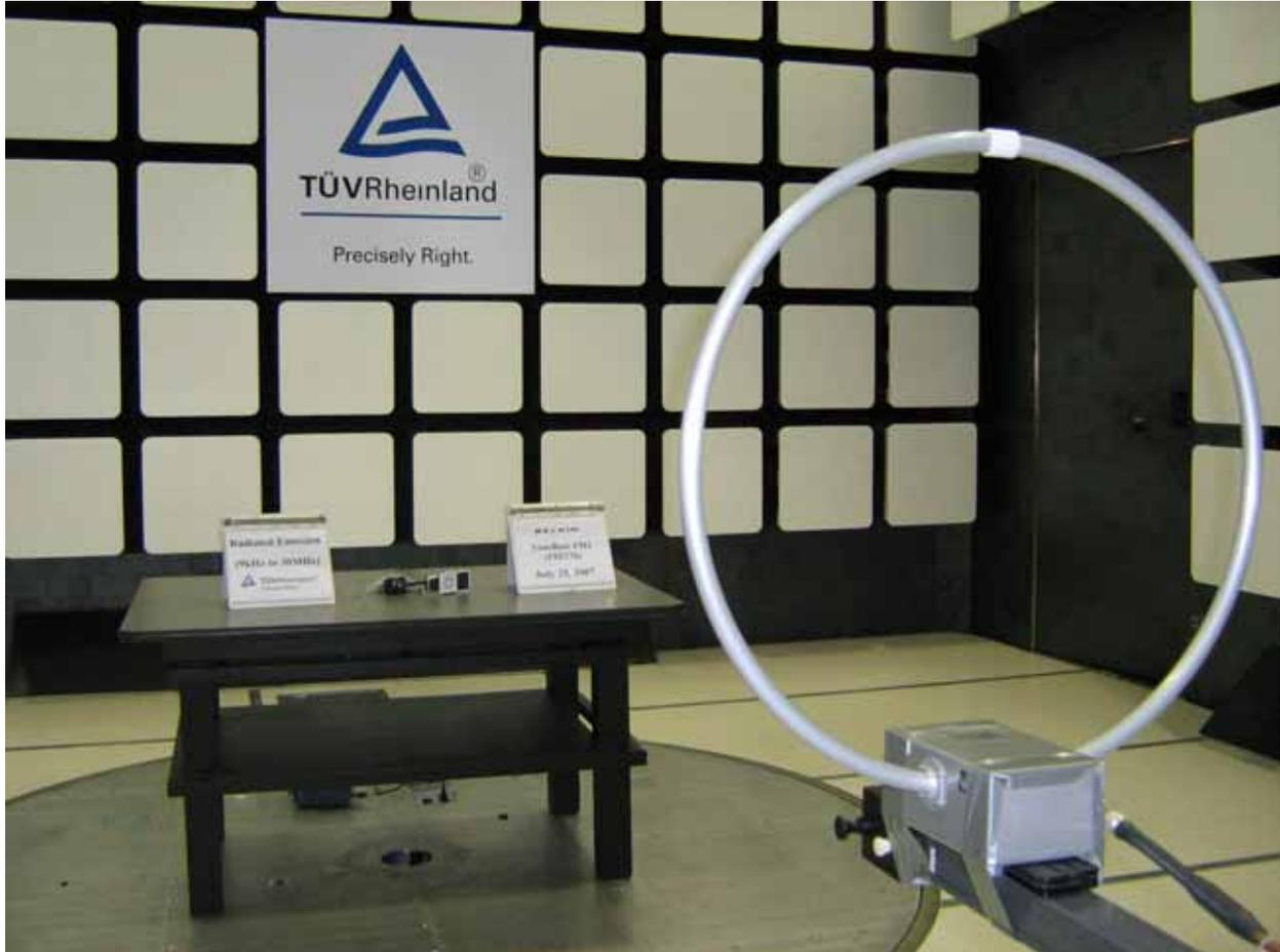
Test Setup: 9 kHz to 30MHz Radiated Emission at 3 Meter Distance – Facing Away
