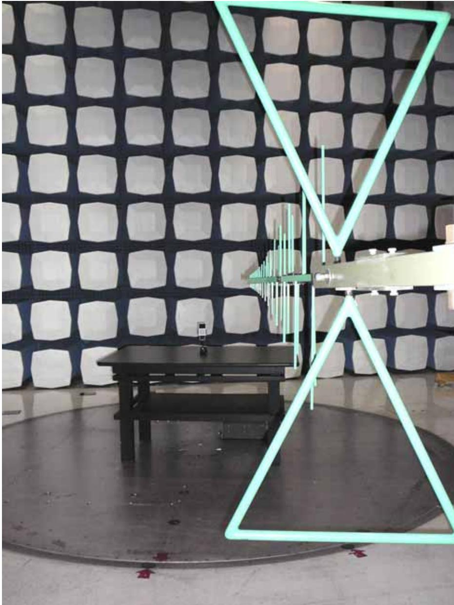
Test Setup: 30MHz to 1000MHz Radiated Emission at 3 Meter Distance – Rear View
