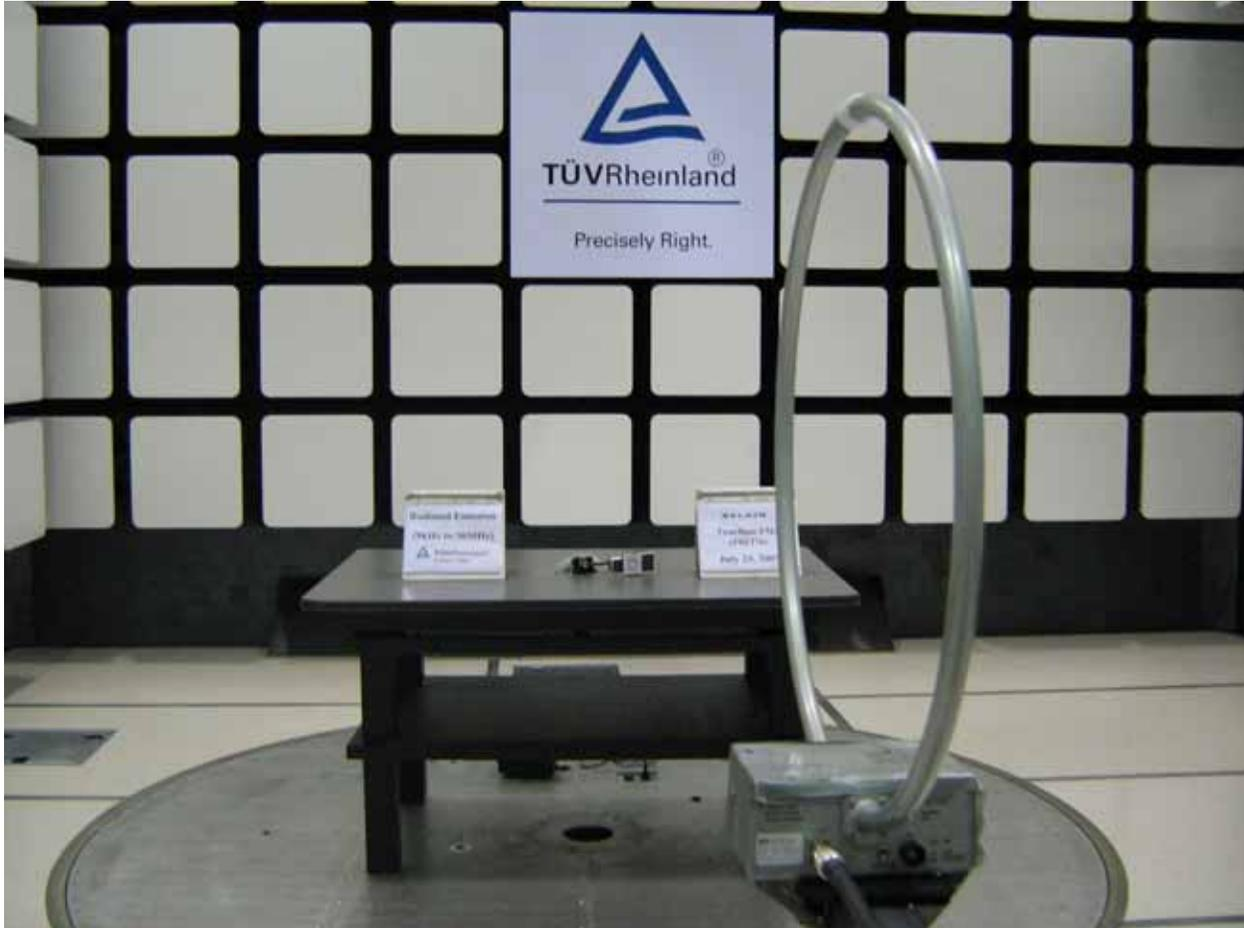
Test Setup: 30MHz to 1000MHz Radiated Emission at 3 Meter Distance – Front View
