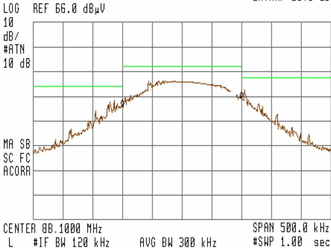
Figure 16 – Bandedge Measurement for Channel 88.1MHz (Vertical) at 15.87VDC
