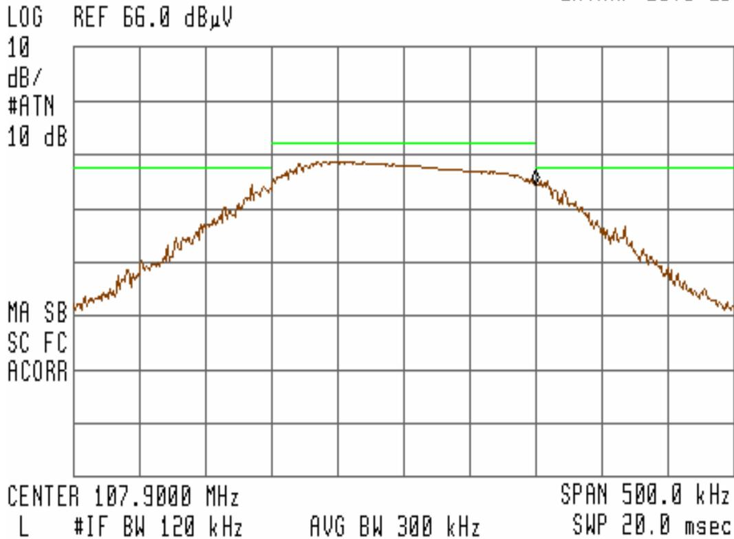
Figure 24 – Bandedge Measurement for Channel 107.9MHz (Vertical) at 15.87VDC
