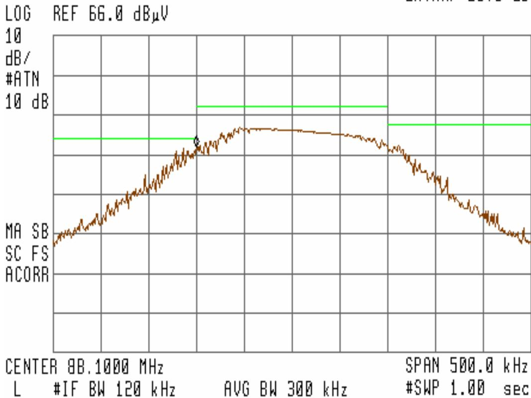
Figure 15 – Bandedge Measurement for Channel 88.1MHz (Vertical) at 11.73VDC
