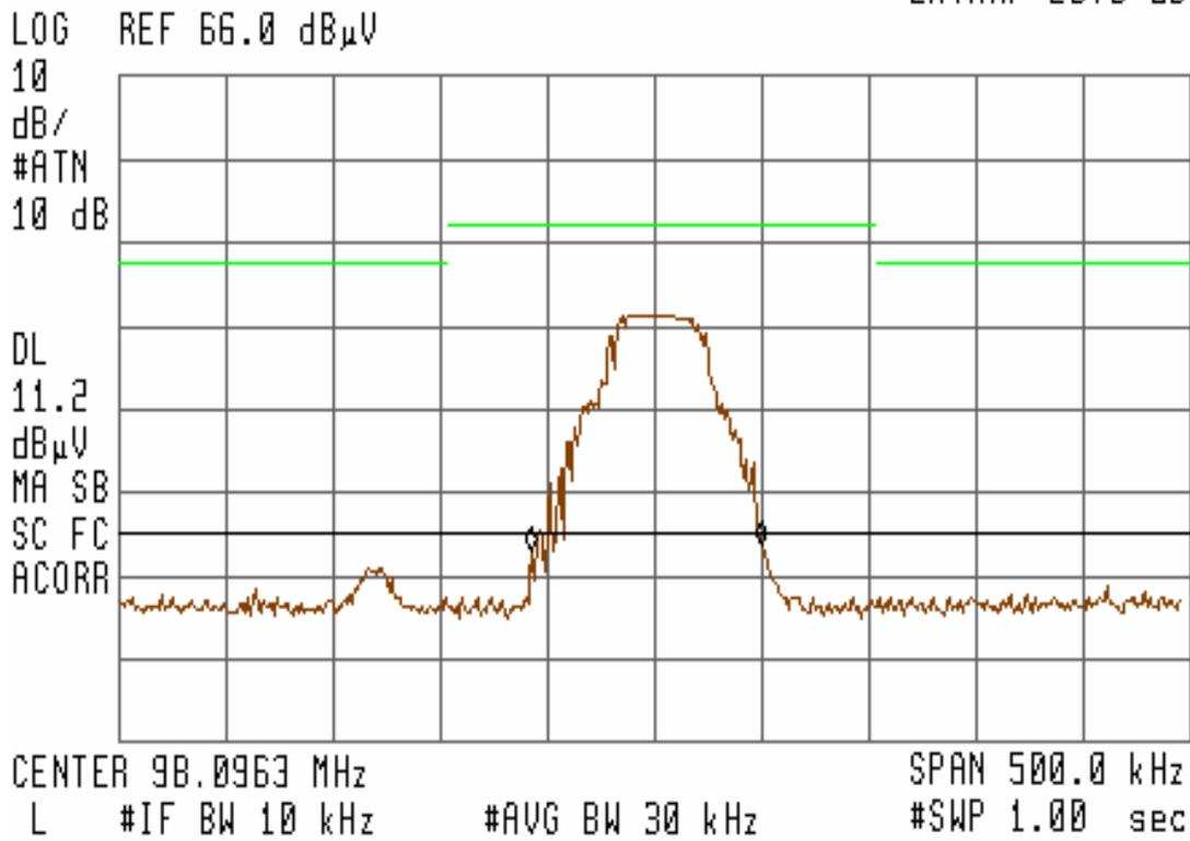
Figure 10 – Channel 98.1MHz (Vertical) – 26dB Bandwidth with 200 kHz Bandwidth Envelope
