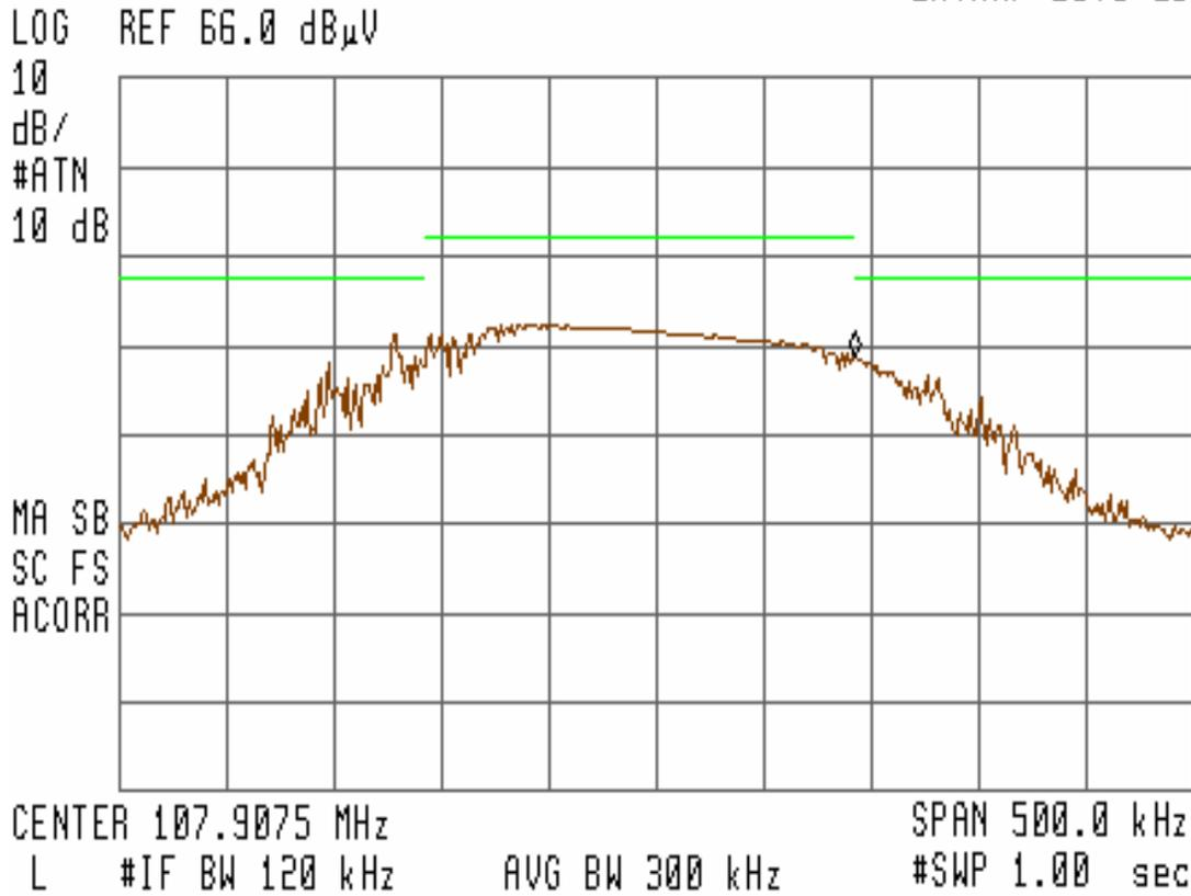
Figure 22 – Bandedge Measurement for Channel 107.9MHz (Horizontal) at 15.87VDC
