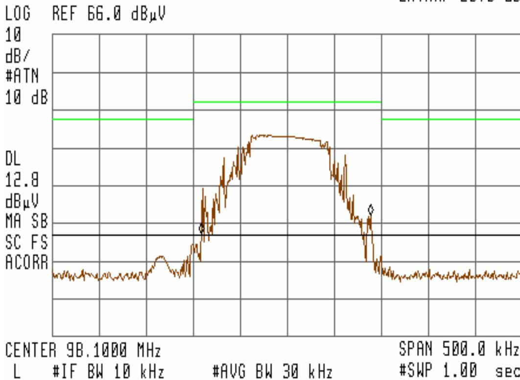
Figure 9 – Channel 98.1MHz (Horizontal) – 26dB Bandwidth with 200 kHz Bandwidth Envelope
