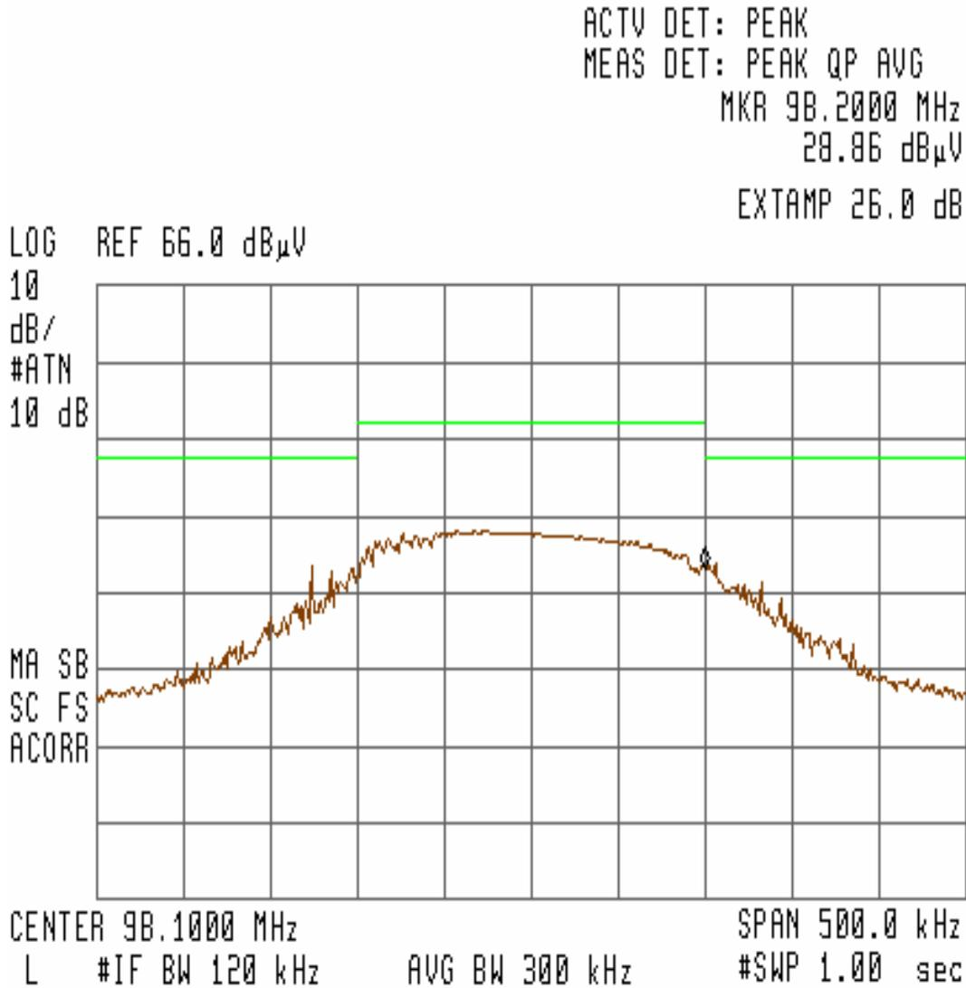
Figure 18 – Bandedge Measurement for Channel 98.1MHz (Horizontal) at 15.87VDC
