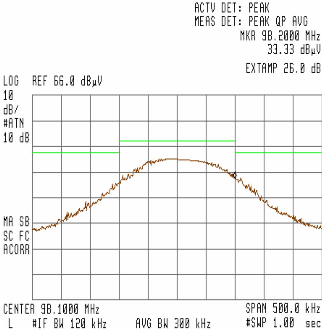
Figure 19 – Bandedge Measurement for Channel 98.1MHz (Vertical) at 11.73VDC
