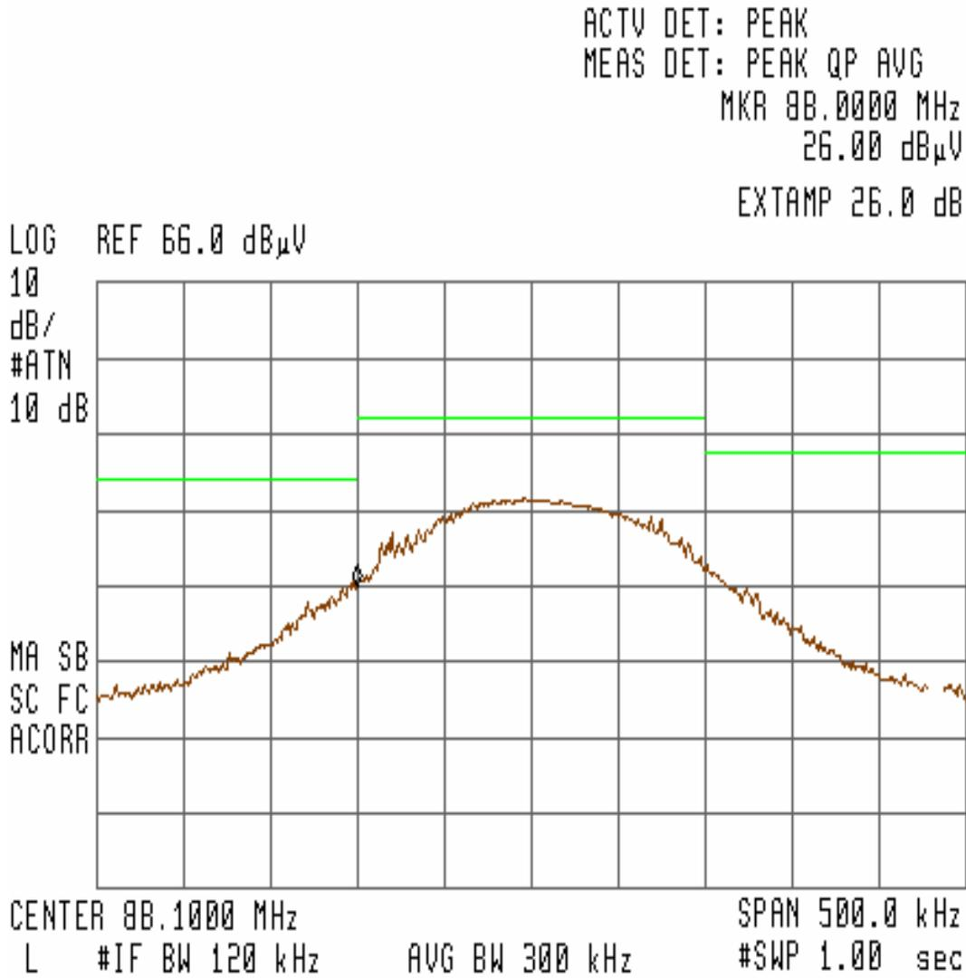
Figure 13 – Bandedge Measurement for Channel 88.1MHz (Horizontal) at 11.73VDC
