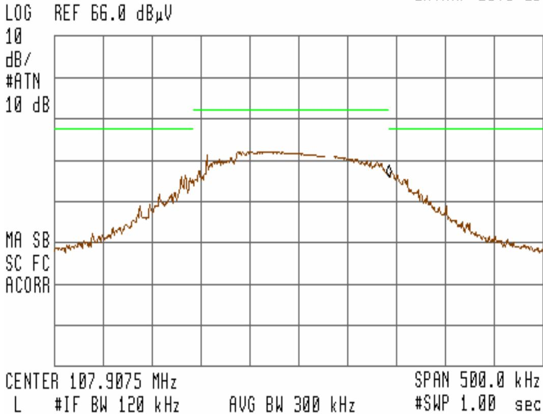
Figure 21 – Bandedge Measurement for Channel 107.9MHz (Horizontal) at 11.73VDC
