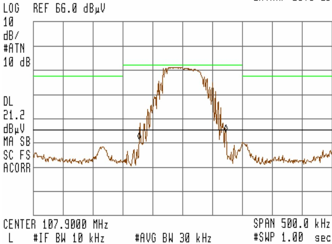
Figure 12 – Channel 107.9MHz (Vertical) – 26dB Bandwidth with 200 kHz Bandwidth Envelope
