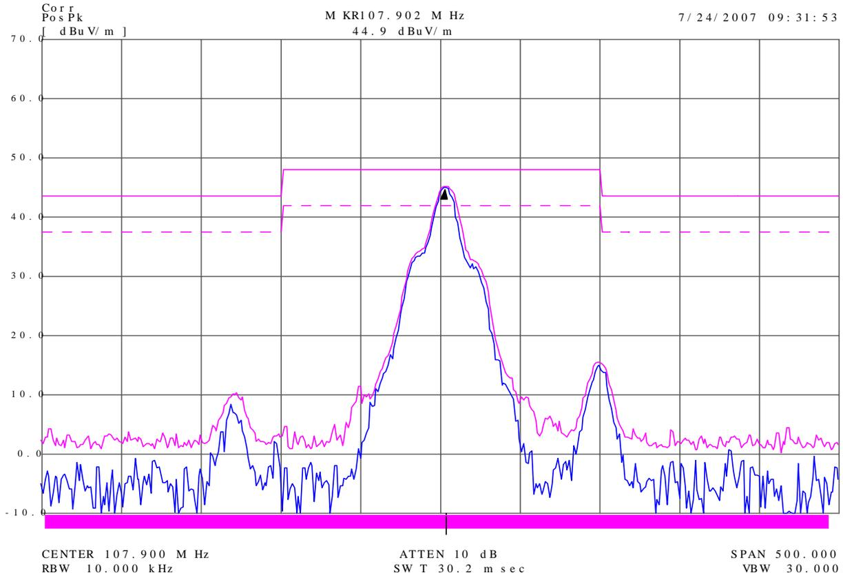
Figure 5 – Channel 107.9MHz Band edge Results for Horizontal
