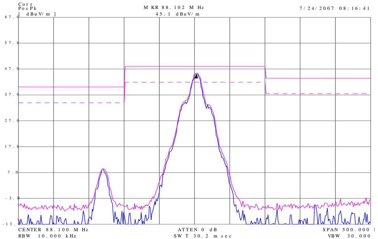
Figure 1 – Channel 88.1 Band edge Results for Horizontal
