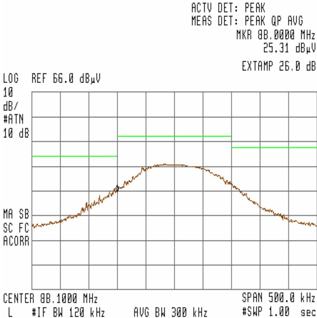
Figure 14 – Bandedge Measurement for Channel 88.1MHz (Horizontal) at 15.87VDC
