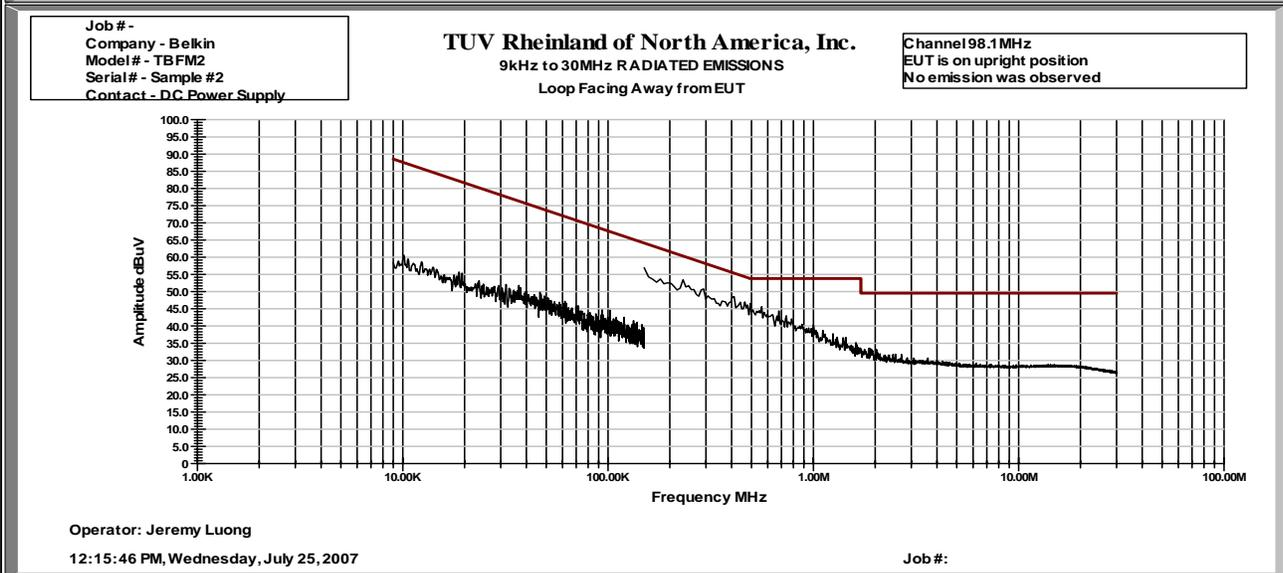
Notes: The fundamental 98.1MHz of the EUT was tested in all three planes and the upright position was worst case. No emission was observed when the loop was facing TBFM2 and facing away.
