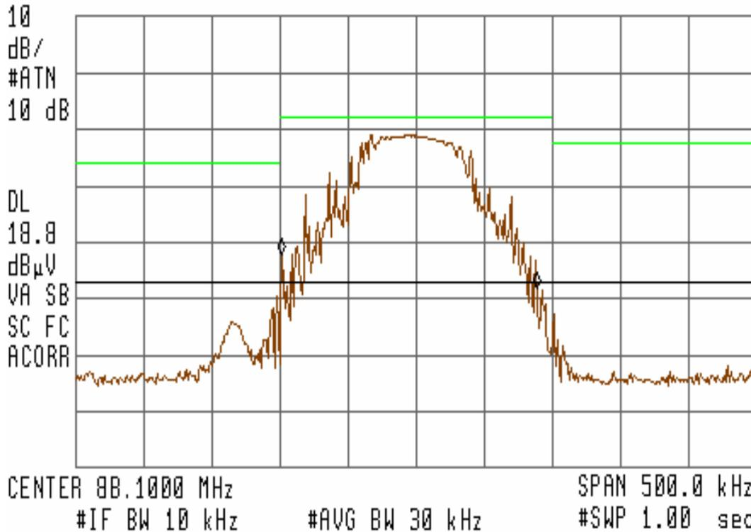
Figure 8 – Channel 88.1MHz (Vertical) – 26dB Bandwidth with 200 kHz Bandwidth Envelope
