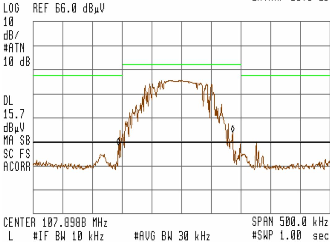
Figure 11 – Channel 107.9MHz (Horizontal) – 26dB Bandwidth with 200 kHz Bandwidth Envelope
