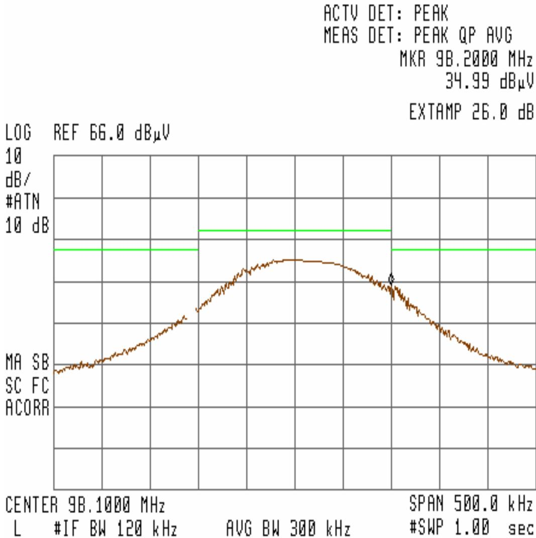
Figure 20 – Bandedge Measurement for Channel 98.1MHz (Vertical) at 15.87VDC
