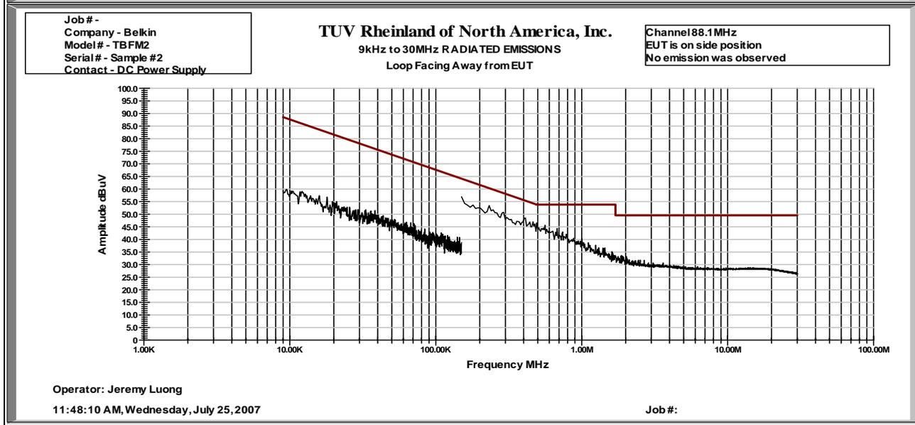
Notes: The fundamental 88.1MHz of the EUT was tested in all three planes and the side position was worst case. No emission was observed when the loop was facing TBFM2 and facing away.
