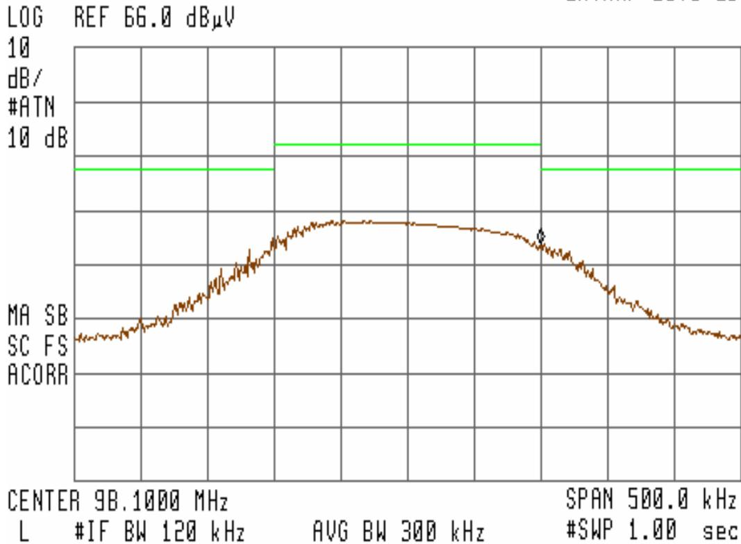
Figure 17 – Bandedge Measurement for Channel 98.1MHz (Horizontal) at 11.73VDC
