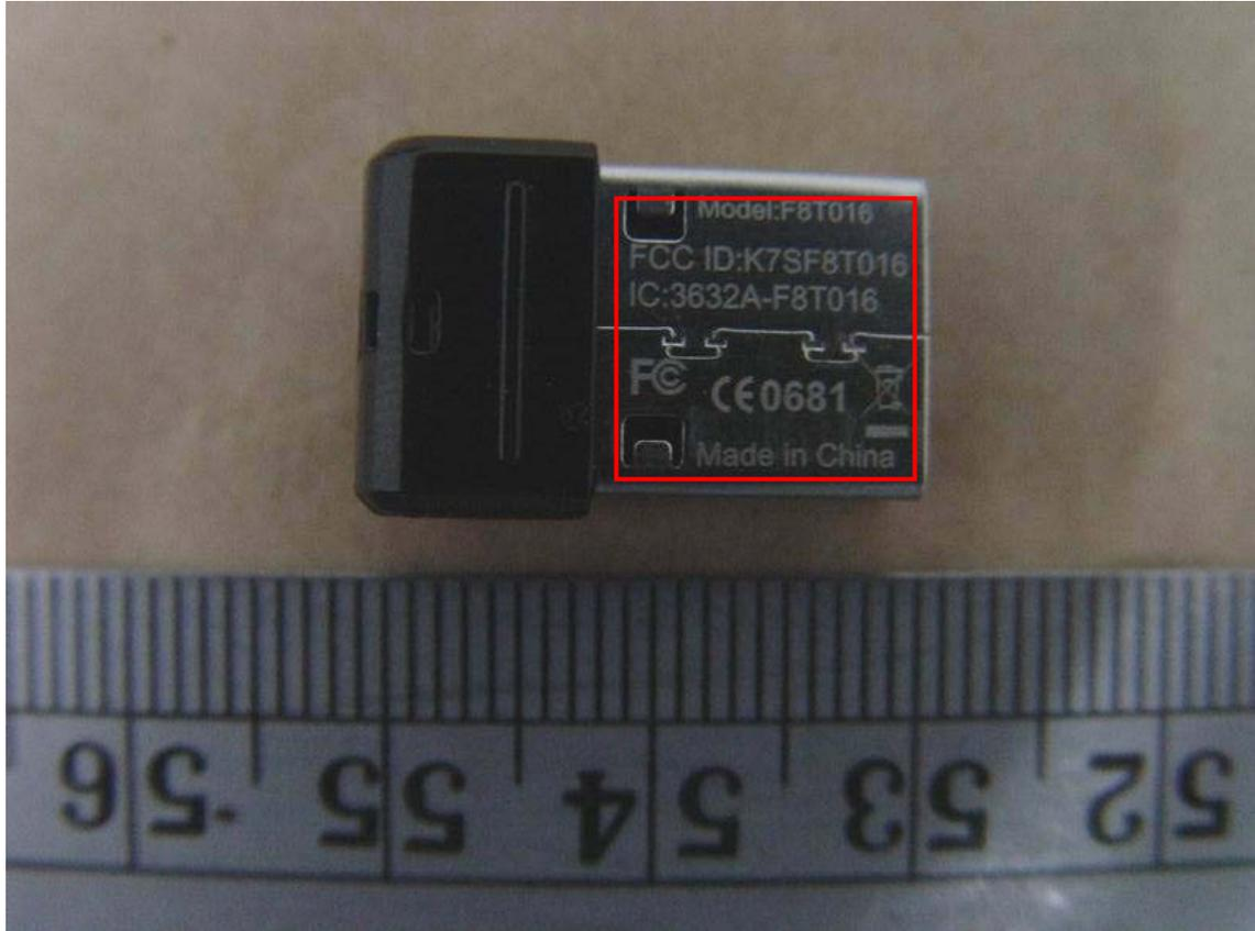
The label size is **8 mm X 8 mm** and because of the size of this device is too small to be placed the other required statement, the following will be placed in the user's manual:
