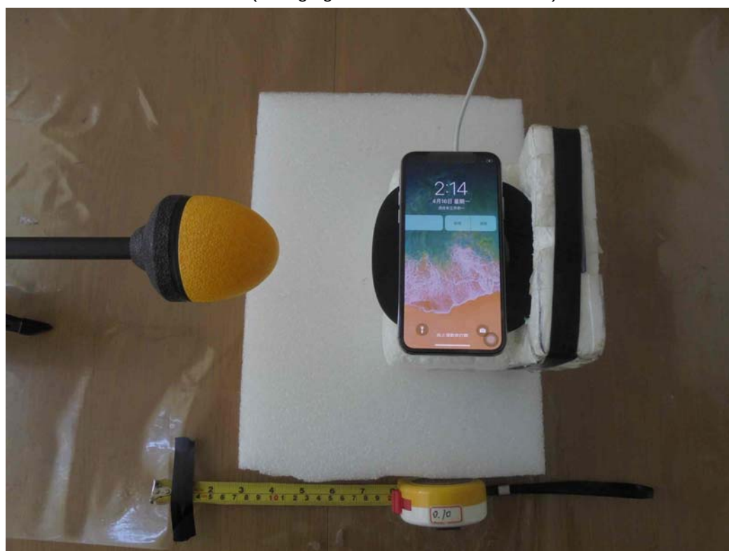
E-Field (Charging Mode with iPhone X - Left)
