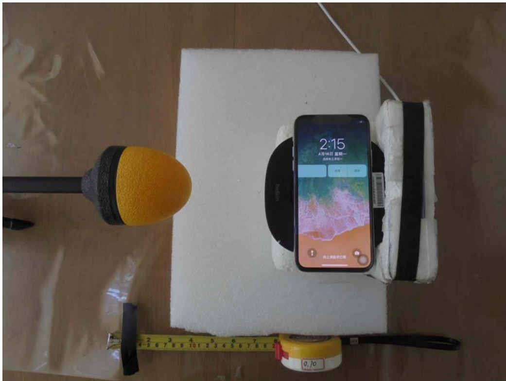
E-Field (Charging Mode with iPhone X - Top)
