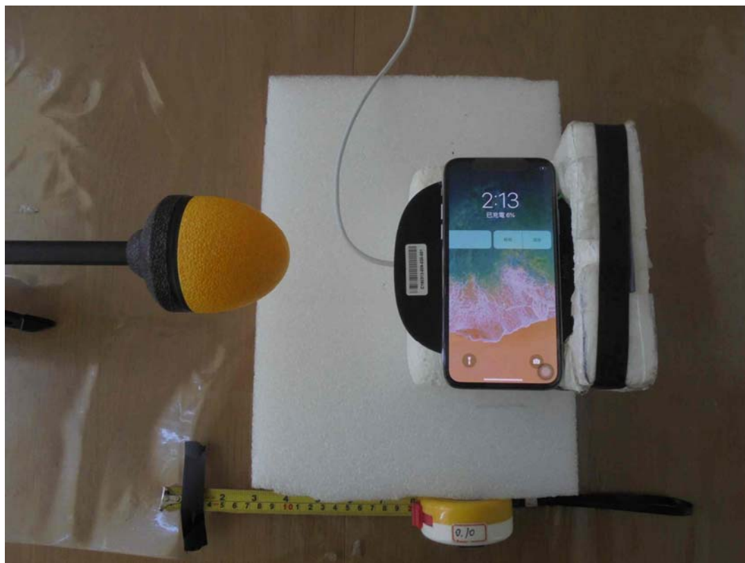
E-Field (Charging Mode with iPhone X - Left)
