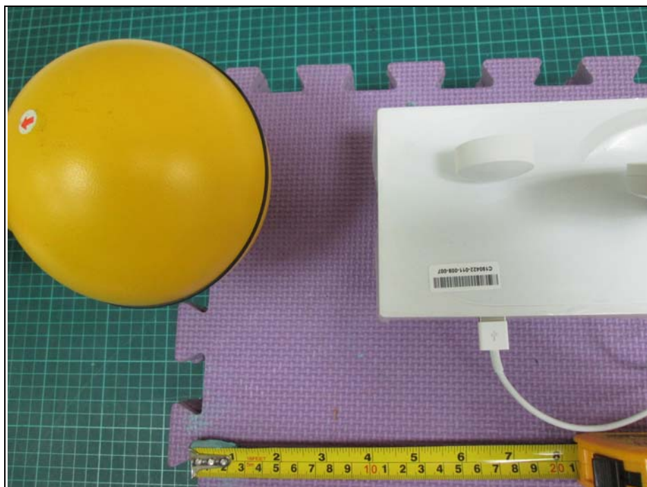
H-Field (Top) (Standby Mode) 15cm
