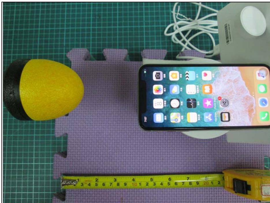
E-Field (Bottom) (Charging Mode) 15cm
