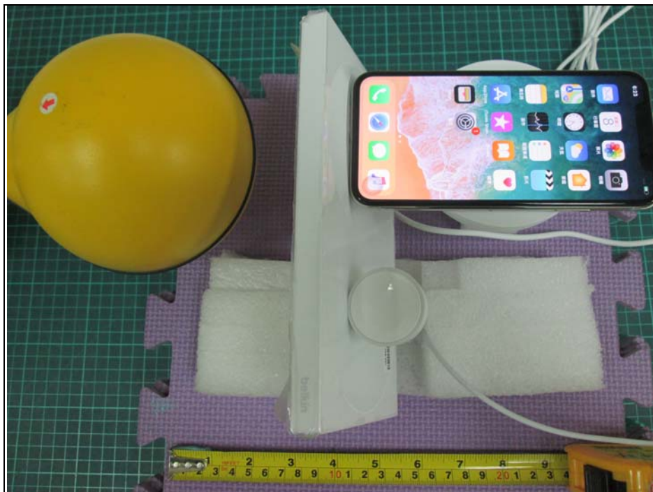
H-Field (Z-axis) (Charging Mode) 20cm
