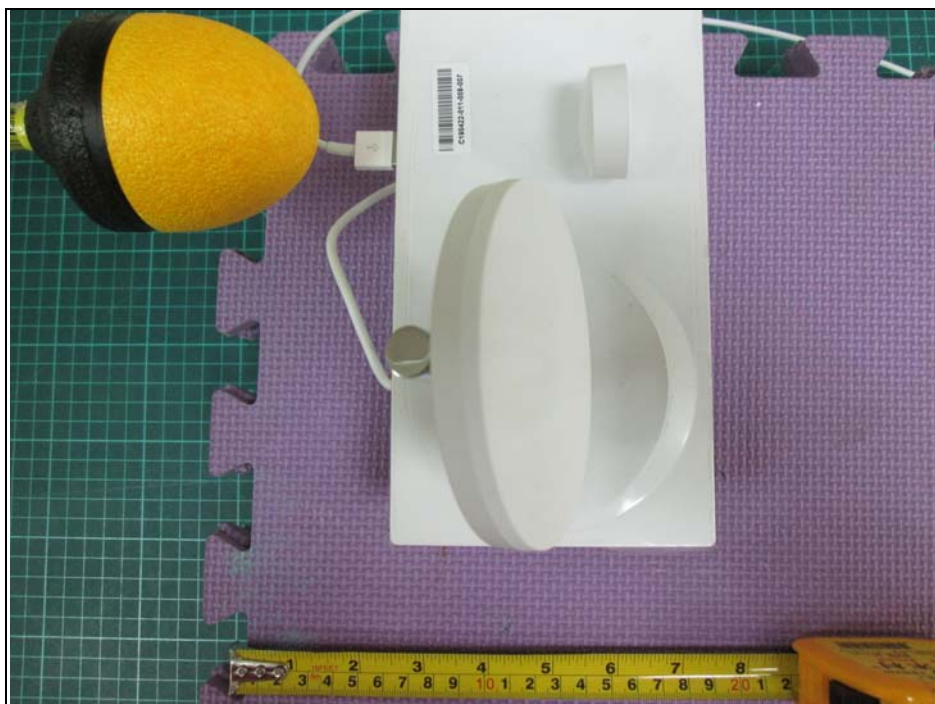
H-Field (Left) (Standby Mode) 15cm
