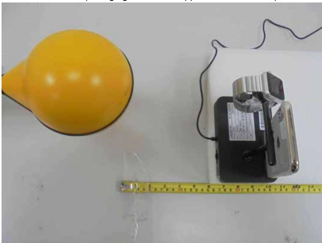
H-Field (Charging Mode with Apple Watch - Bottom)
