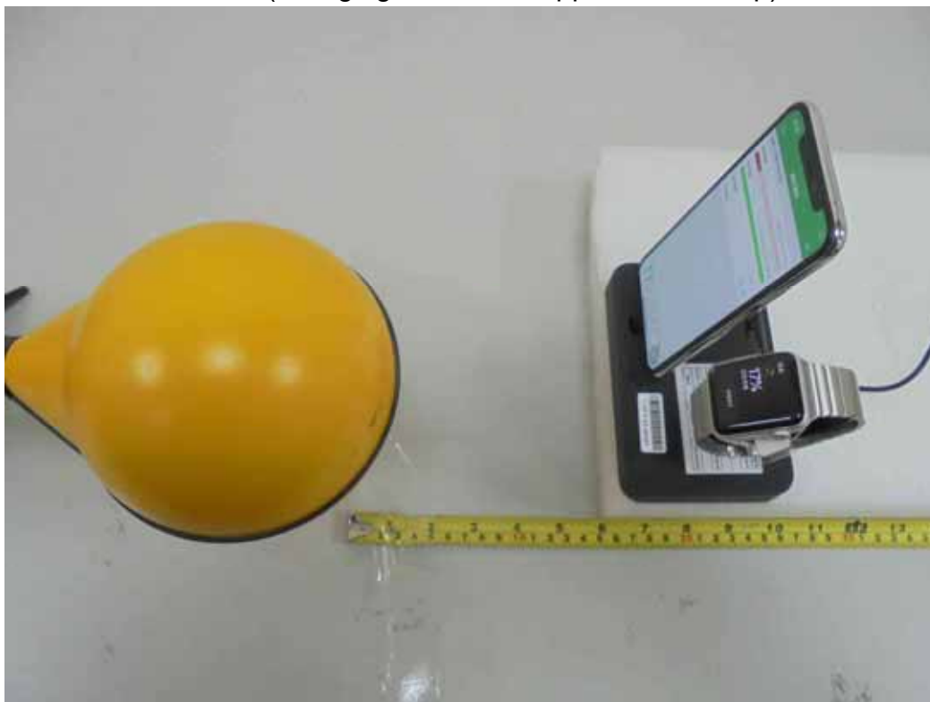
H-Field (Charging Mode with Apple Watch - Bottom)
