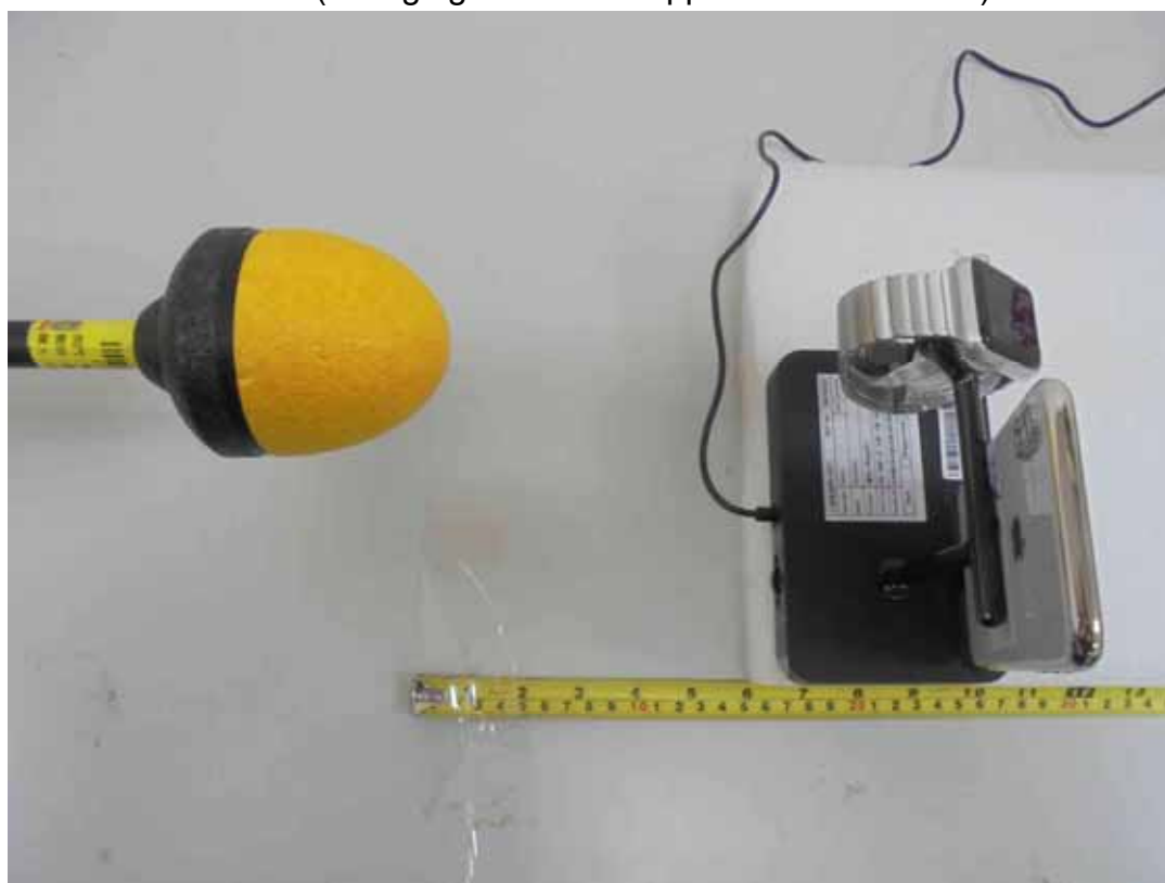
E-Field (Charging Mode with Apple Watch - Bottom)
