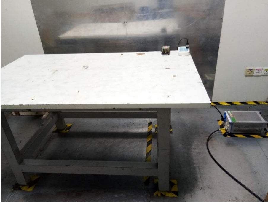
Photos of Power Line Conducted Emission Measurement
