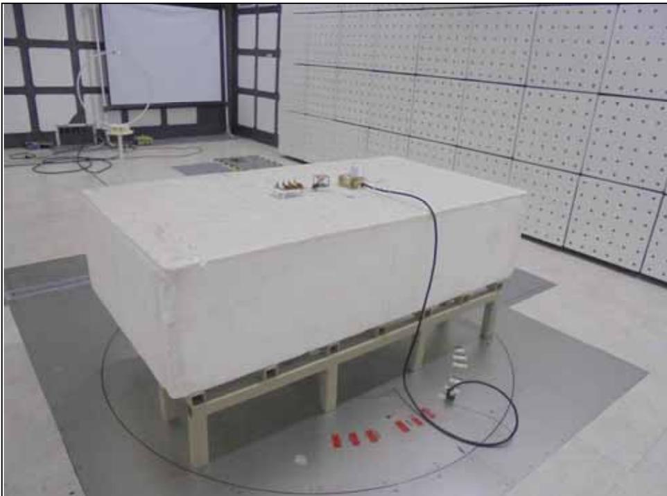
RADIATED EMISSION TEST (Mode B)
