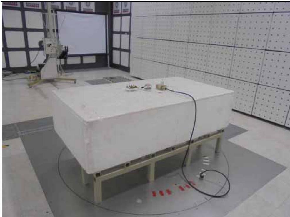
RADIATED EMISSION TEST (Mode B)
