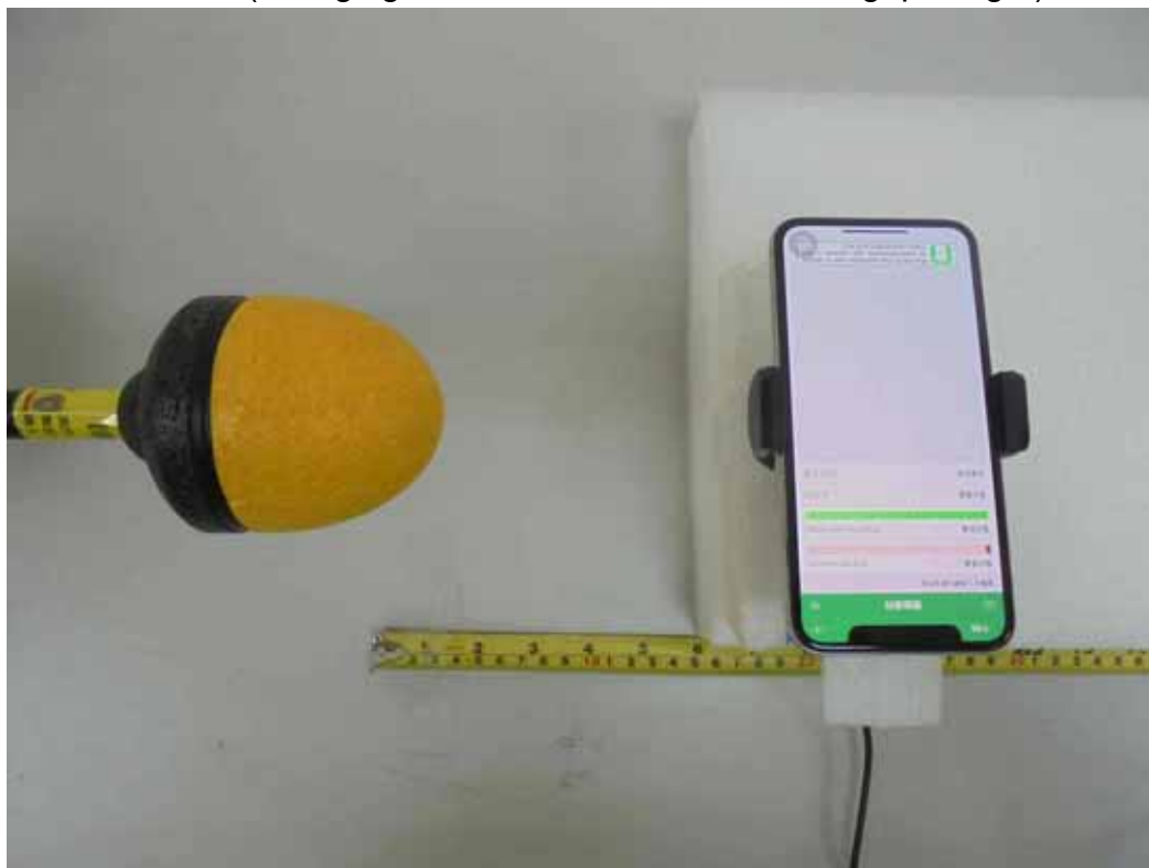
E-Field (Charging Mode with iPhone with 3mm gap - Right)
