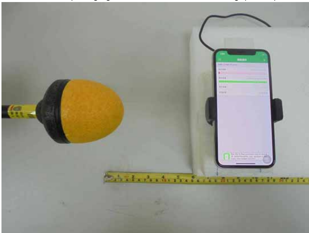
E-Field (Charging Mode with iPhone with 3mm gap - Left)
