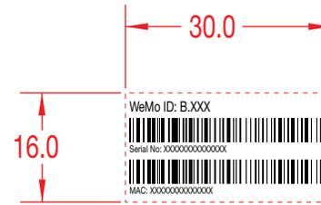
Elements within red boxes are to be printed in BLACK on pre-printed label at the factory.
