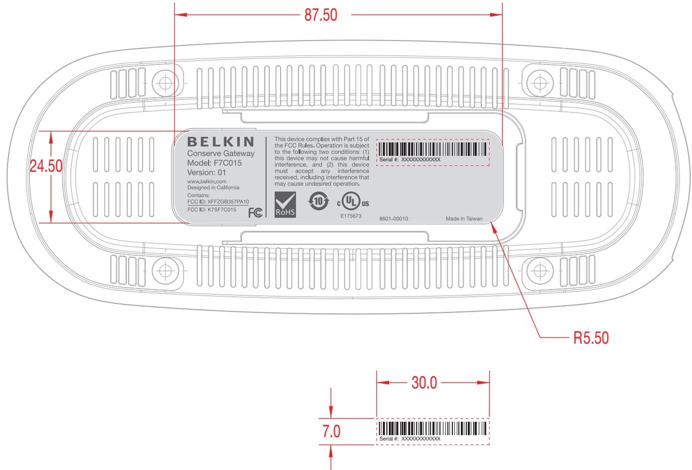
Elements within red boxes are to be printed in BLACK on pre-printed label at the factory.
