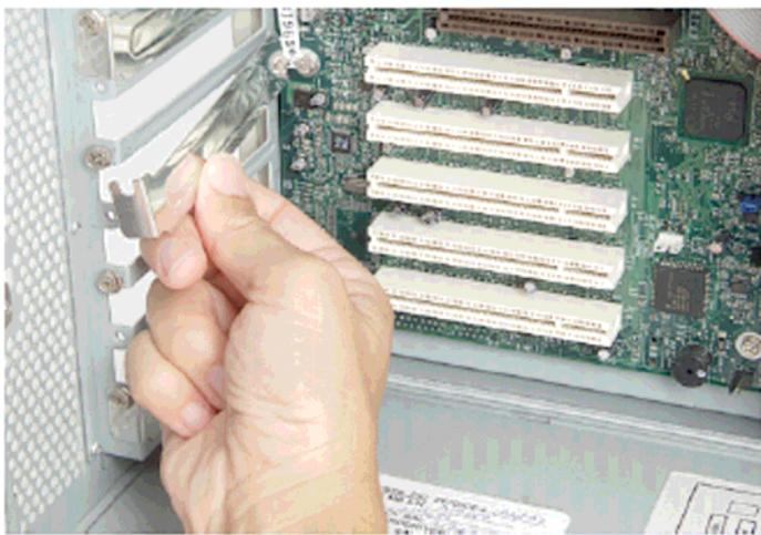
**1B.5** Push the Card firmly into the PCI slot that you have chosen. Apply pressure as needed until the connector is fully seated.
