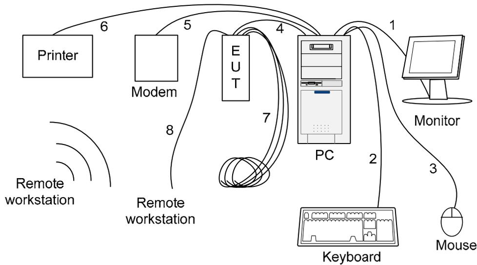
1. The VGA cable is connected from PC to the Monitor.
