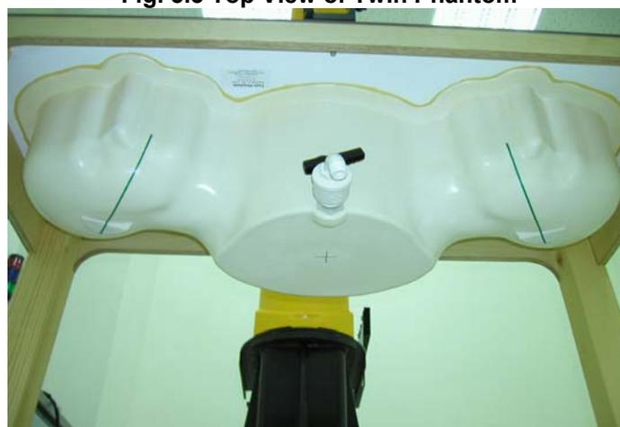
Fig. 5.4 Bottom View of Twin Phantom
