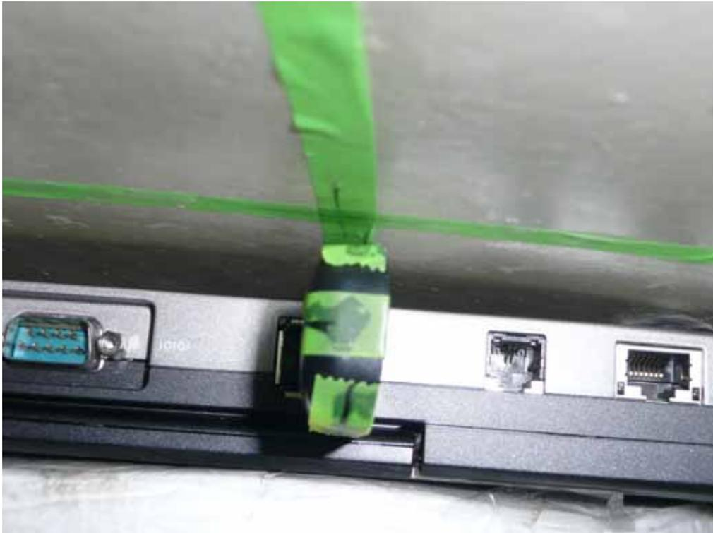
The Vertical-Back of the EUT to the flat phantom distance 5mm.
