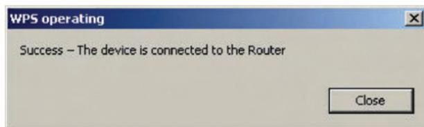
**PIN:** Your notebook computer has an 8-digit PIN that is associated with WPS. Select the WPS-enabled network and click "Connect" to start the WPS process. Choose the PIN-method option and complete the WPS procedure on your router's setup utility.
