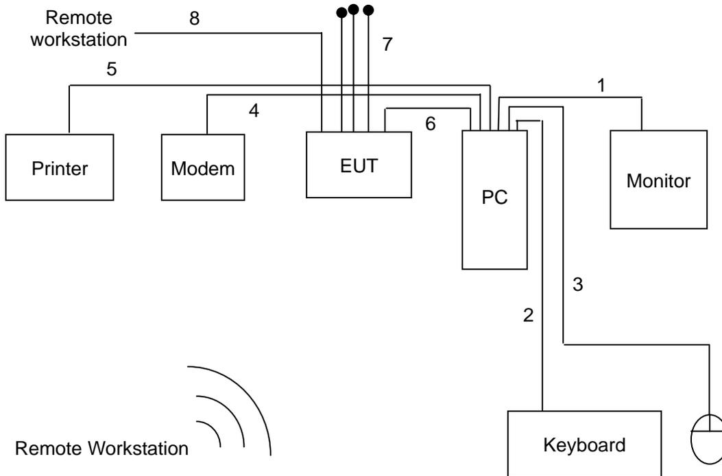
1. The VGA cable is connected from PC to the Monitor.
