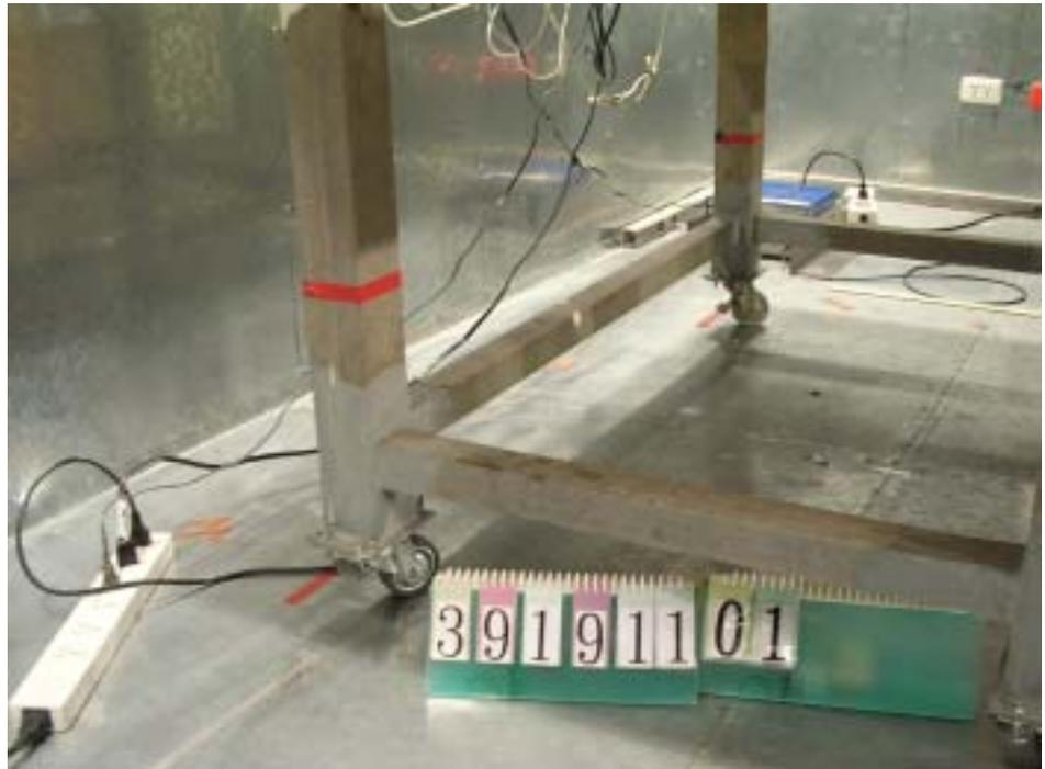
**1.2. Photographs of Radiated Emission Test Configuration**
