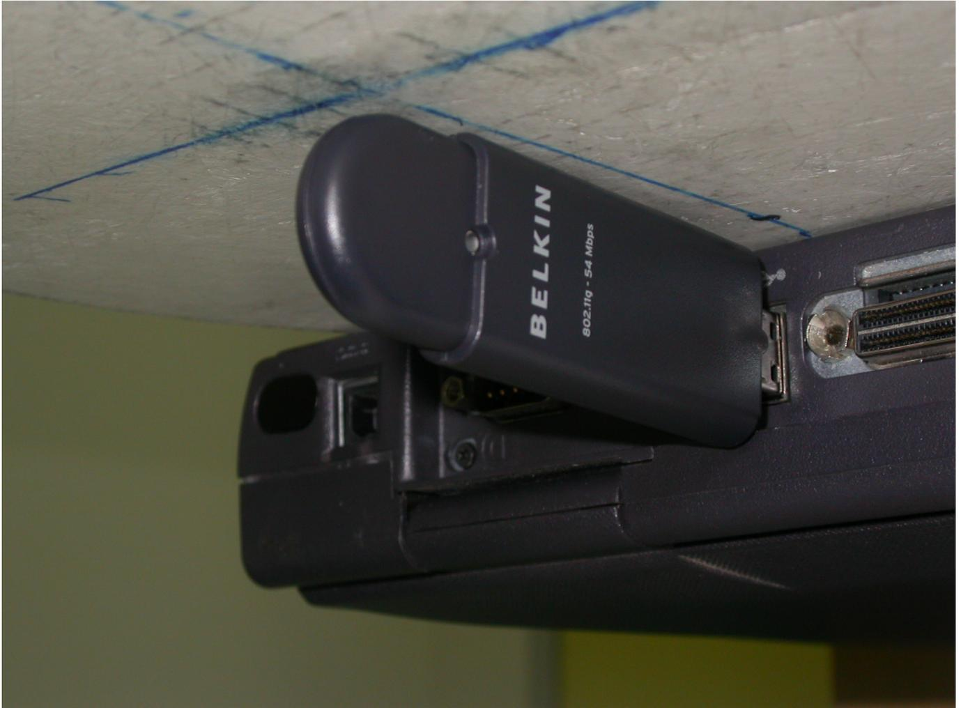
**The Bottom of the EUT to the flat phantom distance 4 mm**
