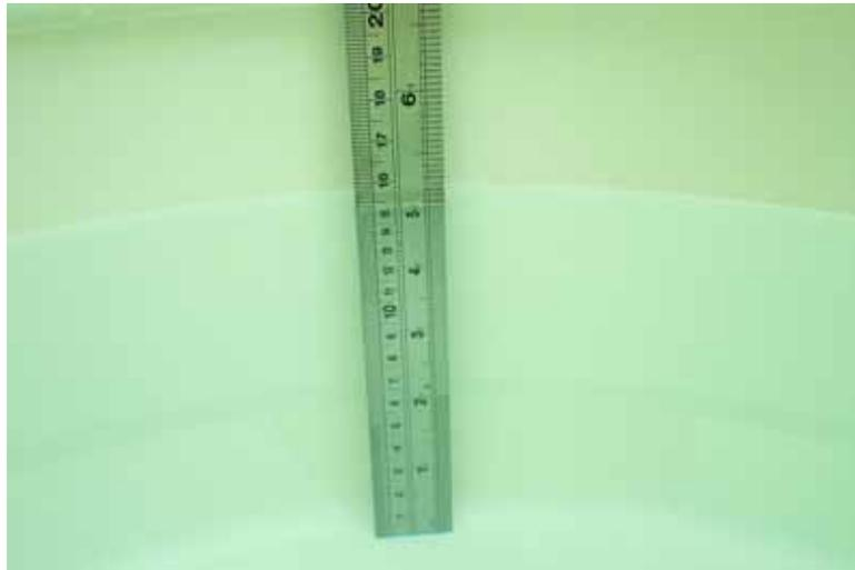
**Fig 6.1 The liquid height from the bottom of the phantom body is 15.2 centimeters**
