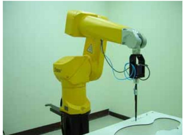
**Fig. 5.2 Probe setup on robot**
