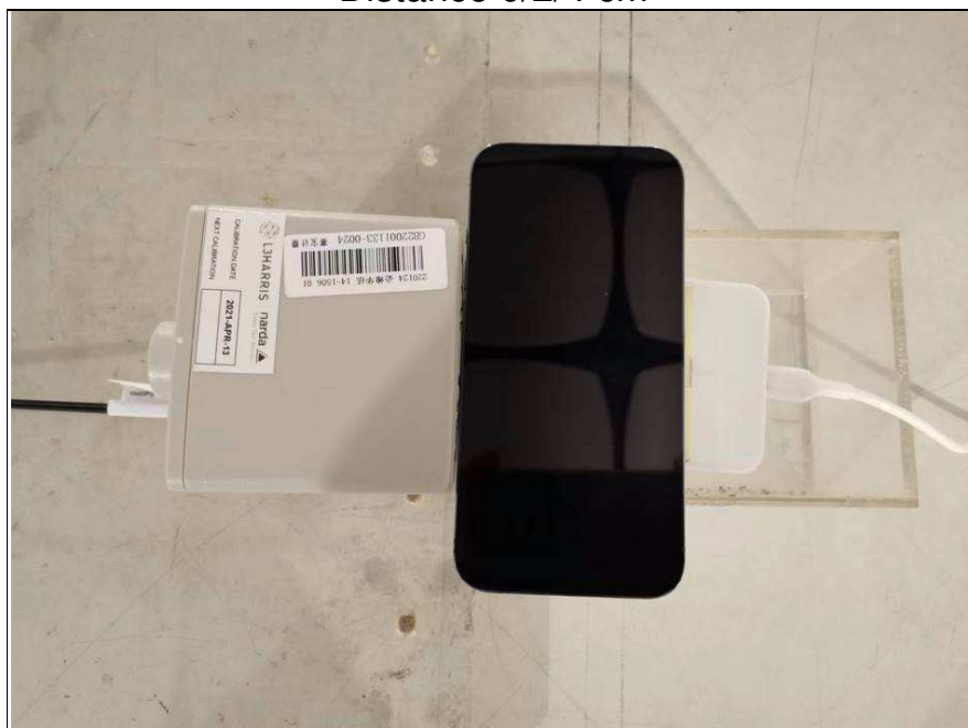
Electric Field & Magnetic Field (Charging mode with iPhone 13 Pro) Distance 0/2/4 cm
