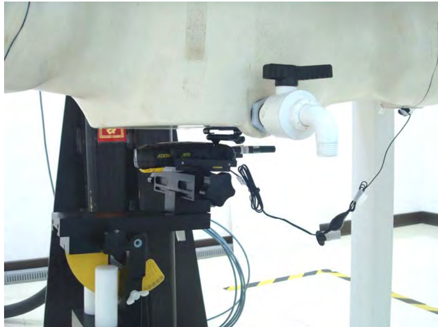
Figure 18. EUT with Headset and Belt clip
