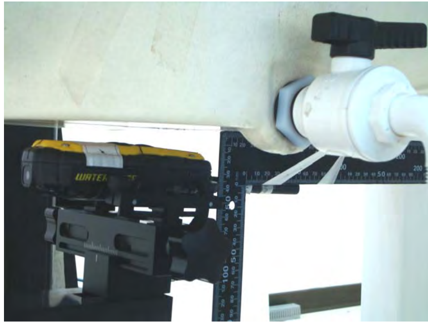
Figure 16. EUT Face to Phantom 15 mm spacing
