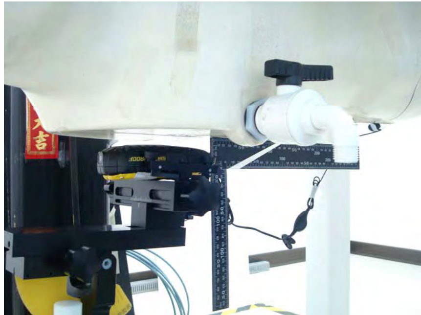
Figure 17. EUT with Headset to Phantom 15 mm spacing
