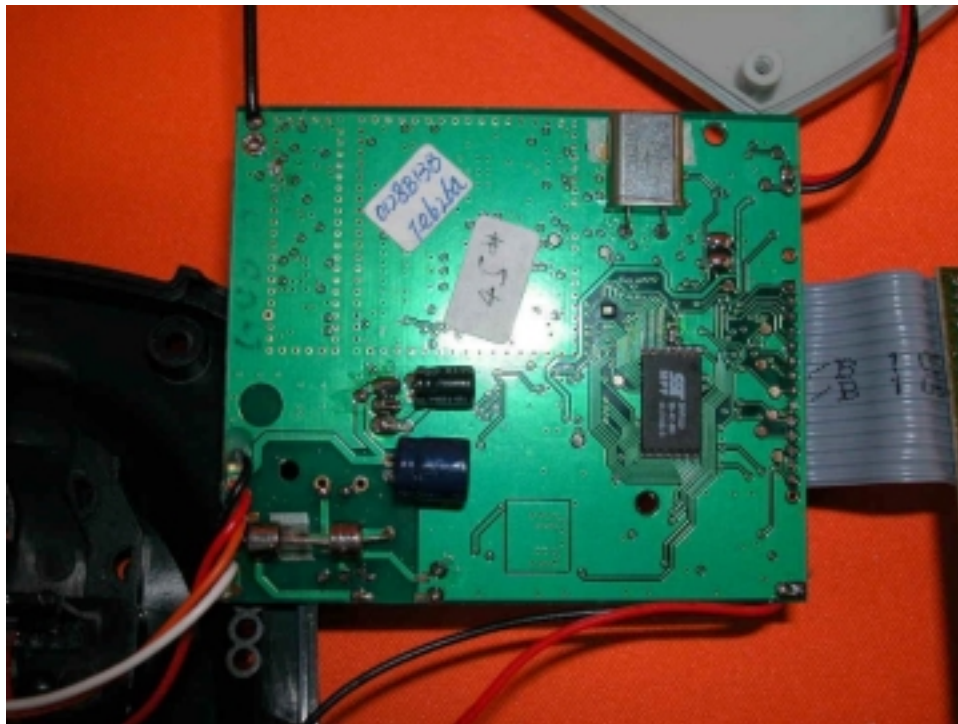
Base Oscillator PCB solder side
