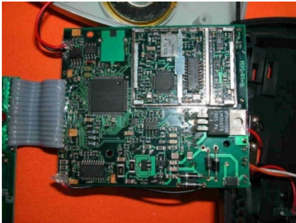
Base Oscillator PCB comp side
