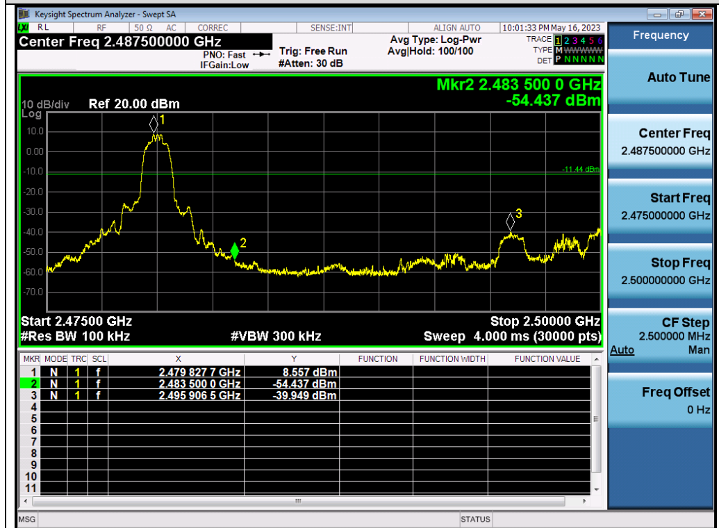
Test_Graph_EDR_ANT1_2480_3Mbps_Higher Band Edge Emissions
