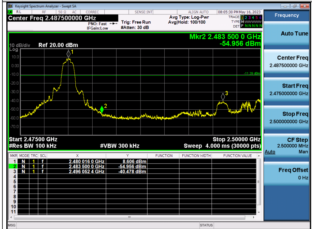
Test_Graph_EDR_ANT1_2480_2Mbps_Higher Band Edge Emissions
