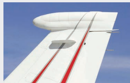
The AMT-700 is typically housed under a tail-mounted radome, but can also be mounted at several locations on the fuselage.
