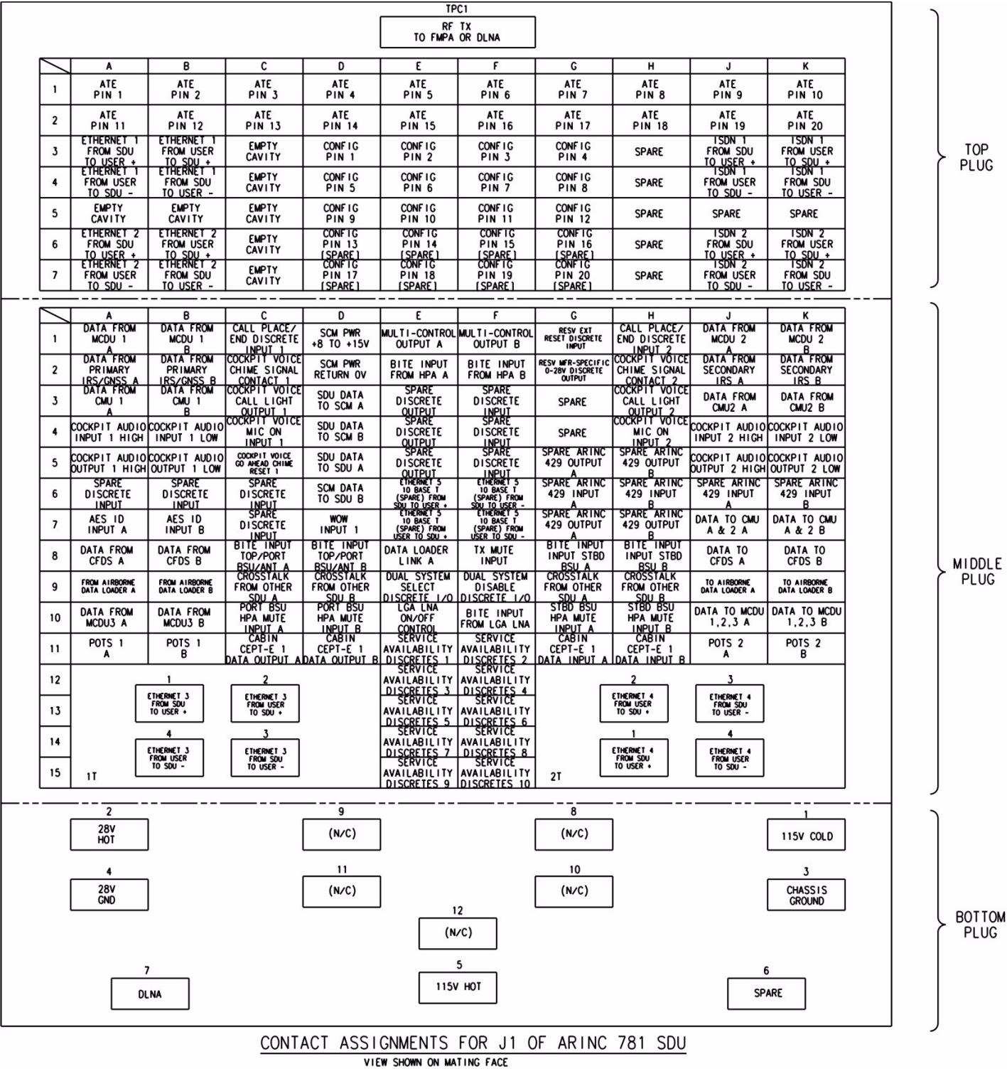
Figure 3-9 ARINC 781 System Interconnect Drawing, 1394-B-1001 Rev A00 (Sheet 3 of 3)
