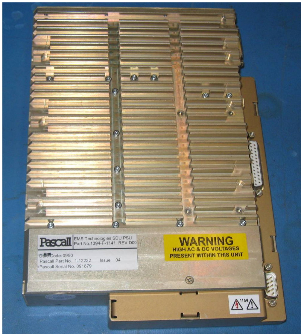
Figure 14: 1394-F-1141 SDU Power Supply Top
