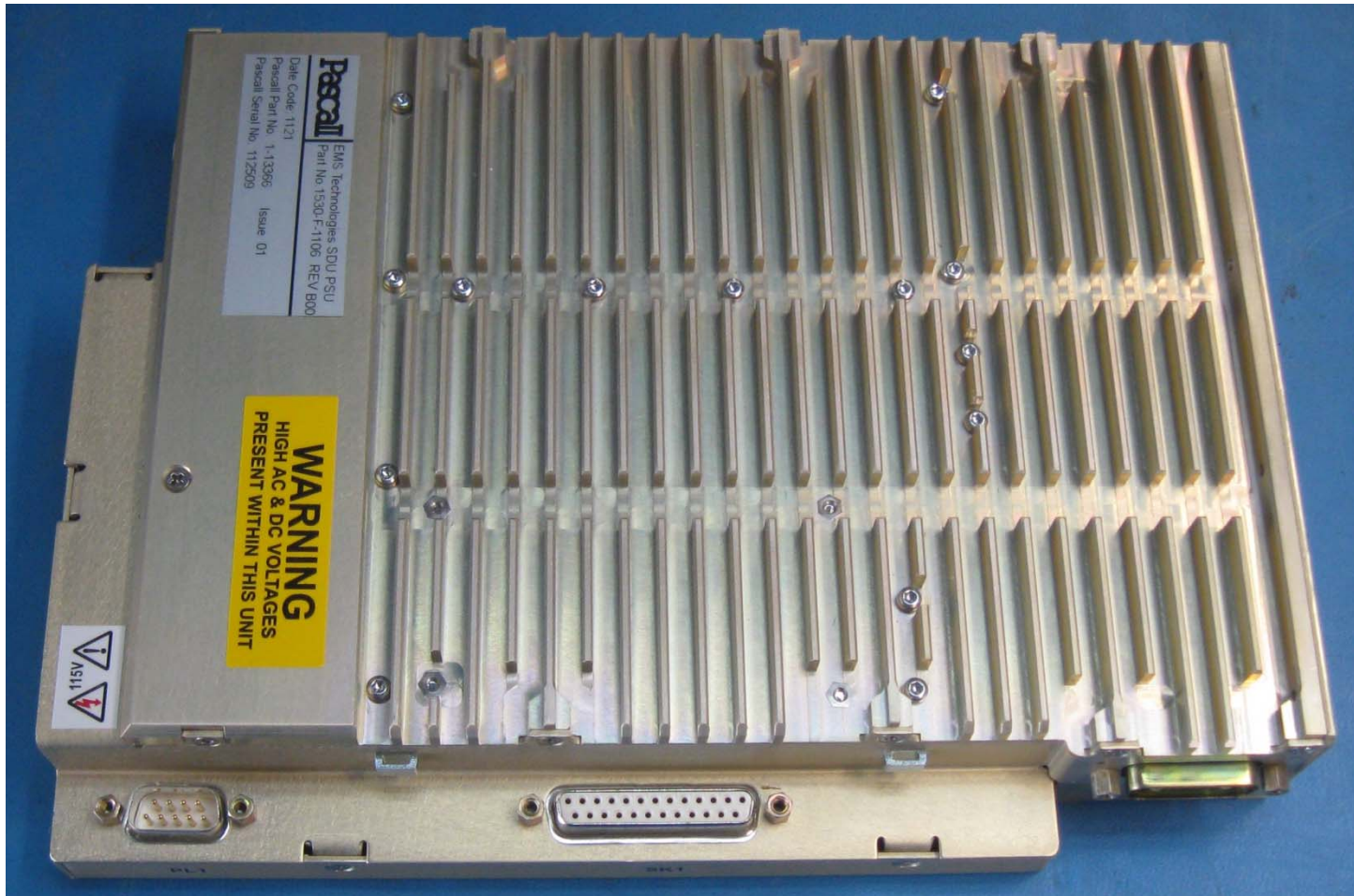
Figure 15: 1530-F-1106 Power Supply Top
