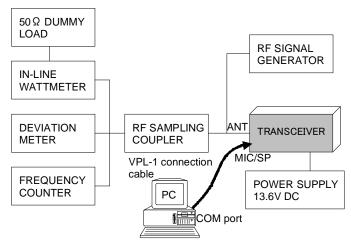
The transceiver must be programmed for use in the intended system before alignment is attempted. The RF parameters are loaded from the file during the alignment process.
