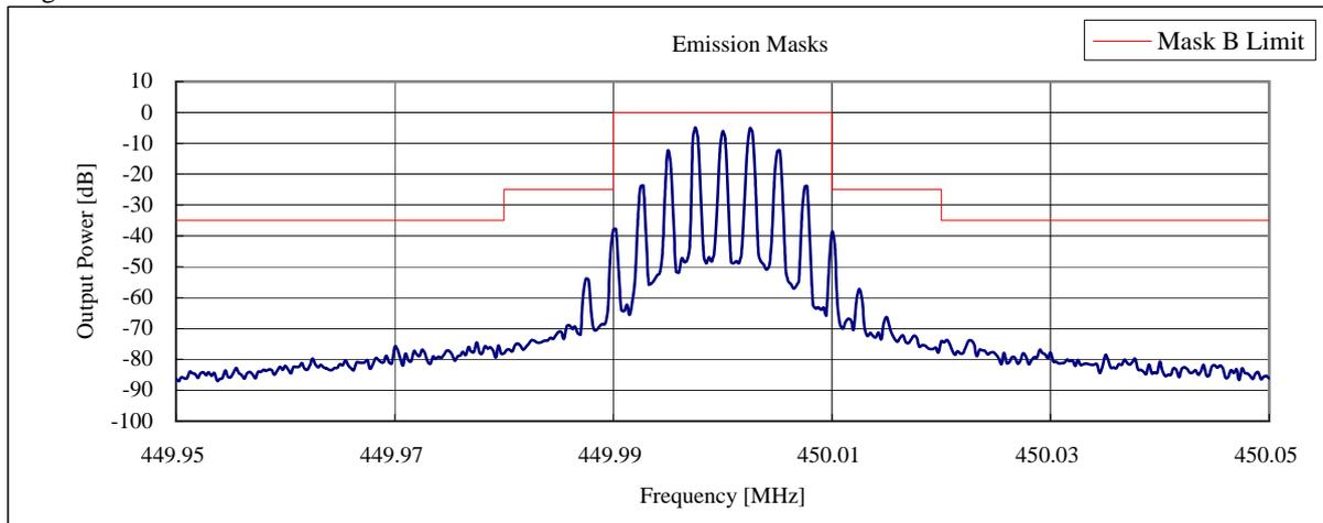
State : Low Power / None Modulation:FM / 450.00 MHz
