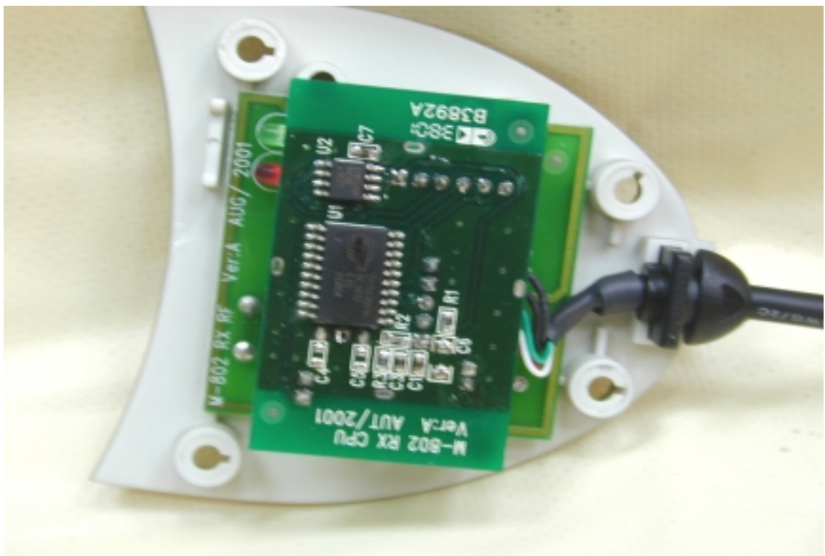
PHOTO. 6. EUT (Model RM-802 Receiver) COMPONENT SIDE VIEW
