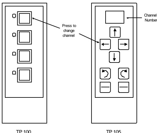
5. To change the channel on a TP 100, press and release the top button and cycle through channels until the desired channel is displayed. For the TP 105, press the left arrow button to change channels.
