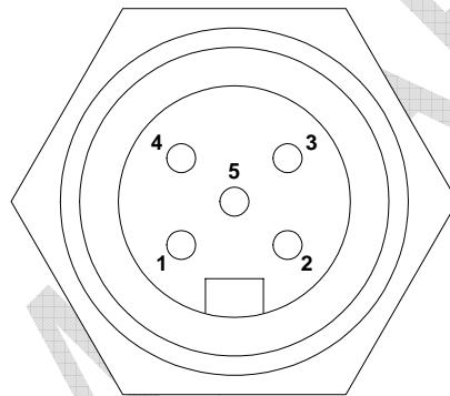
The Wireless CAN Bridge provides factory test functions via a sealed micro style connector (labeled "Auxiliary"). This connector is not used during normal operation.
