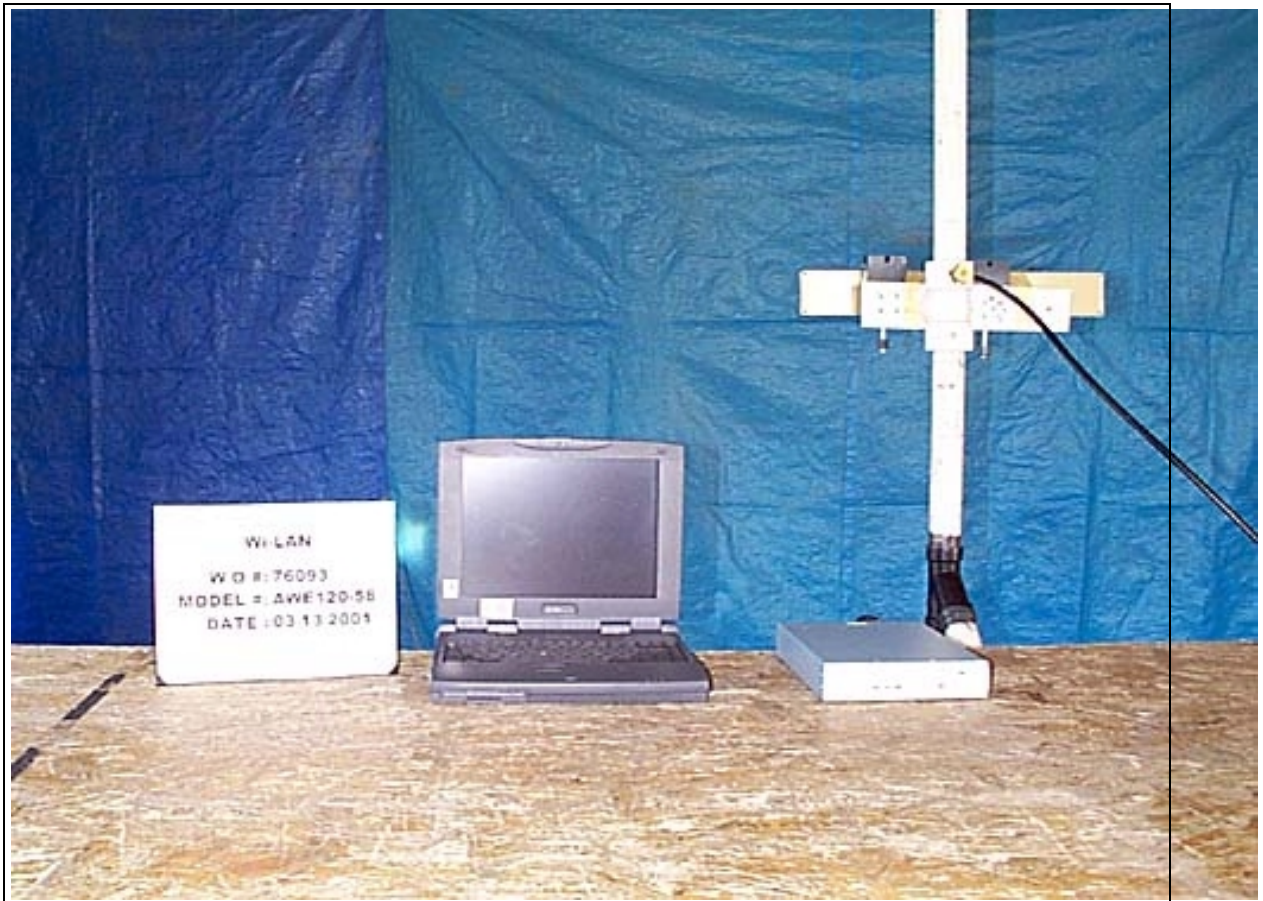
Radiated Emissions Front View (Antenna 2)
