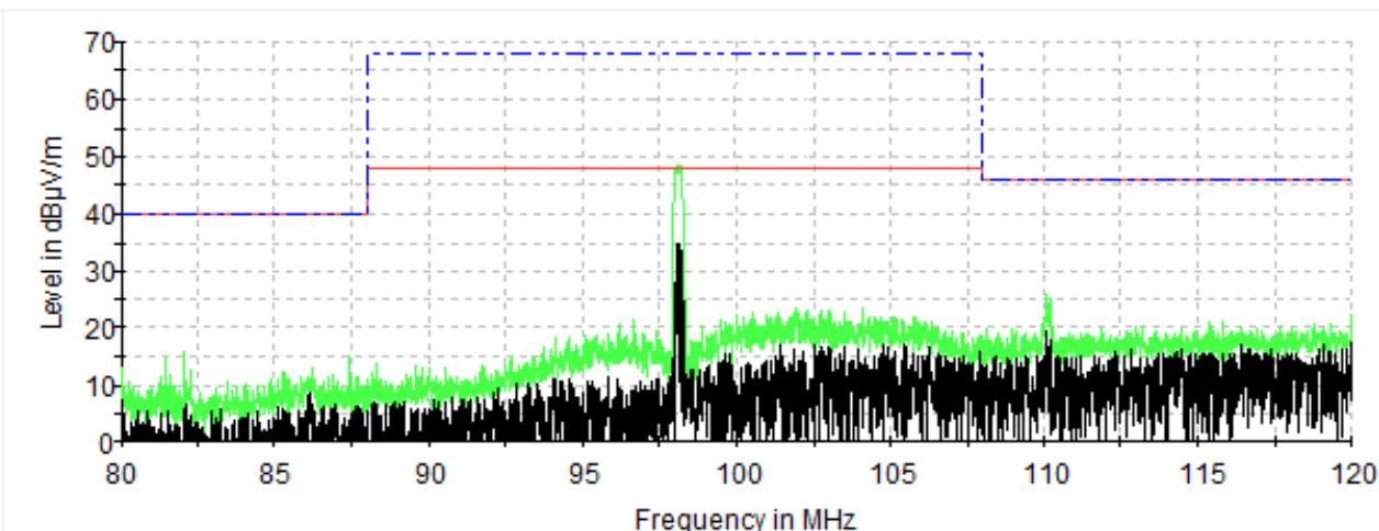
**High Channel, Band Edges: Vertical**
