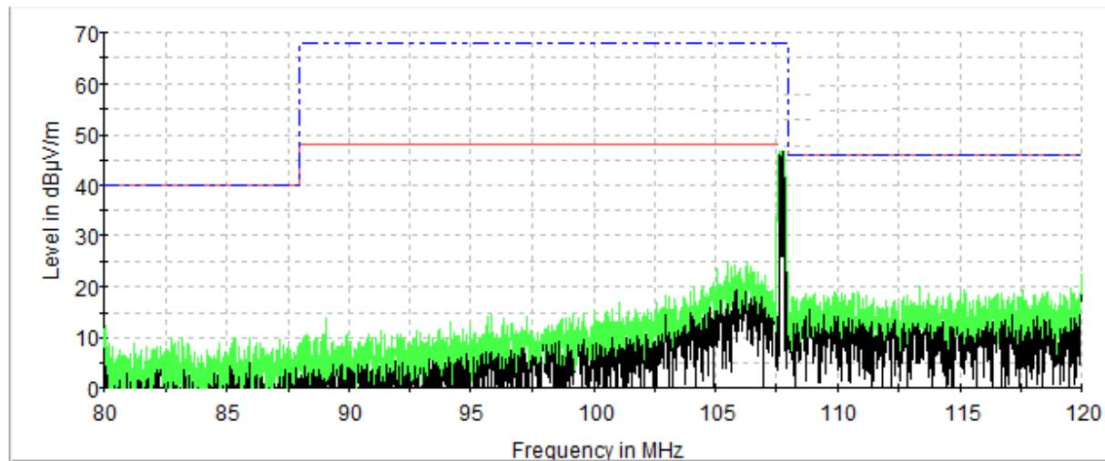
**Band Edge and Field Strength of the Fundamentals**
