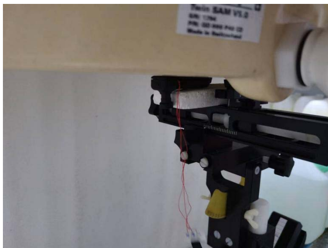
Fig-4.1 Front Face of EUT with 0 cm Gap (Head Mode)
