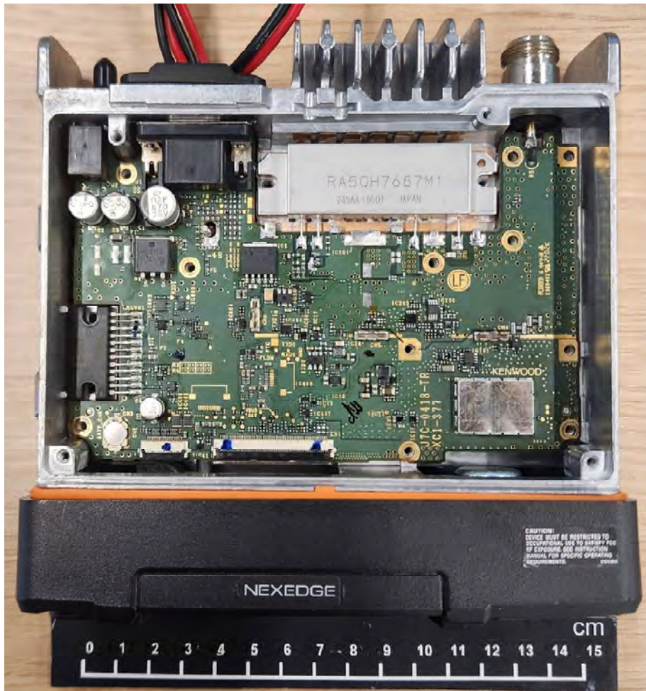
Top Internal View of TX-RX Unit
