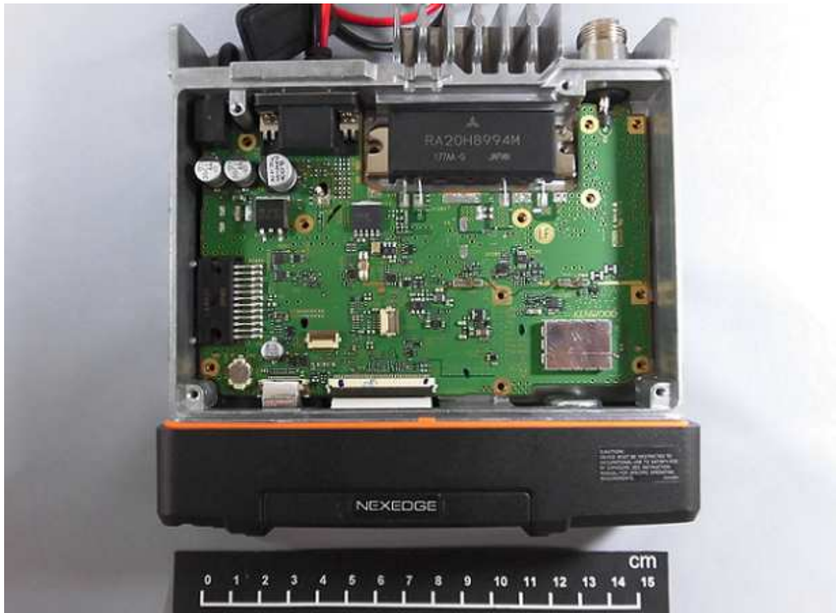
Top Internal View of TX-RX Unit
