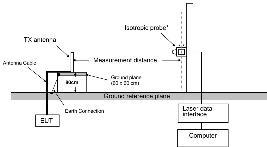
\* : The Isotropic probe position was Vertical orientation from the Ground reference plane from 0.1m to 2m (10cm increments) .
