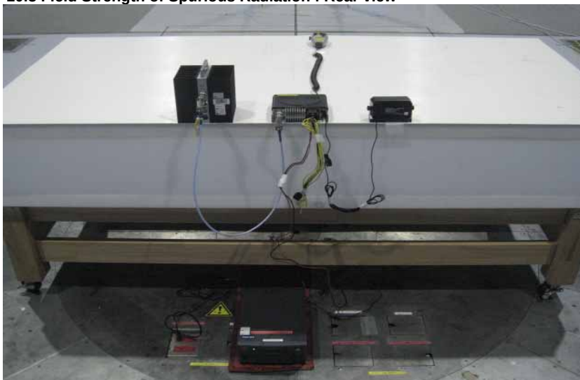
10.3 Field Strength of Spurious Radiation : Rear view
