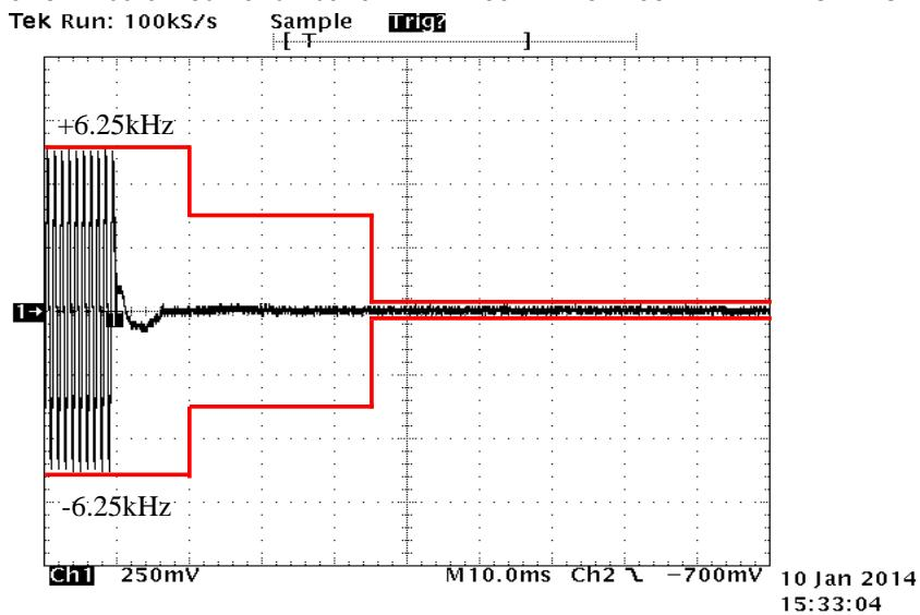
State : High Power / Authorized Bandwidth 6 kHz / 4K00F2D / 511.95 MHz / PTT:ON -OFF
