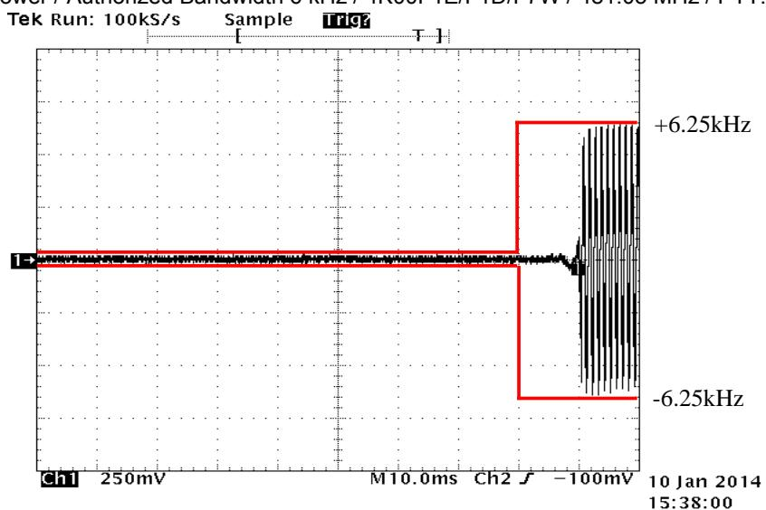
State : High Power / Authorized Bandwidth 6 kHz / 4K00F2D / 511.95 MHz / PTT:OFF -ON
