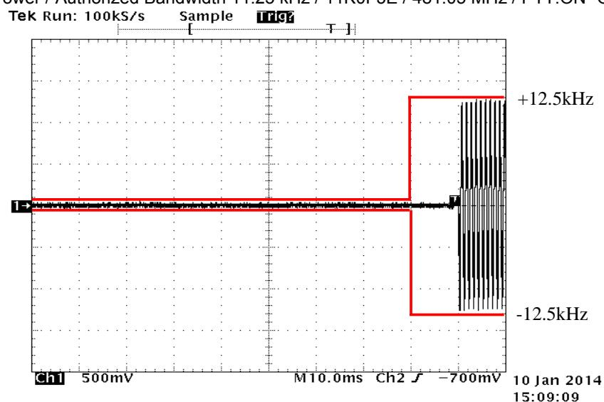
State : High Power / Authorized Bandwidth 6 kHz / 4K00F1E/F1D/F7W / 481.05 MHz / PTT:OFF -ON
