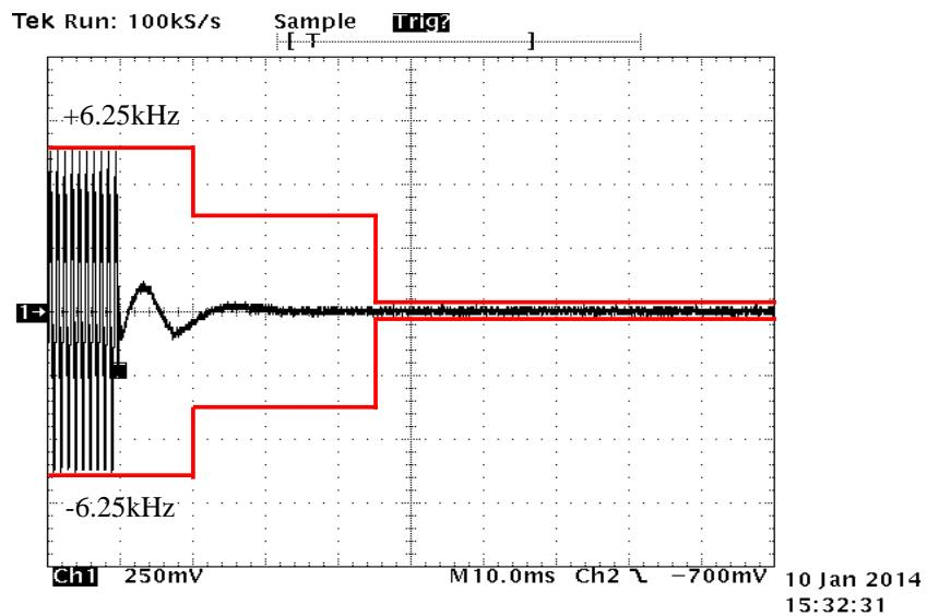
State : High Power / Authorized Bandwidth 6 kHz / 4K00F1E/F1D/F7W / 481.05 MHz / PTT:ON -OFF
