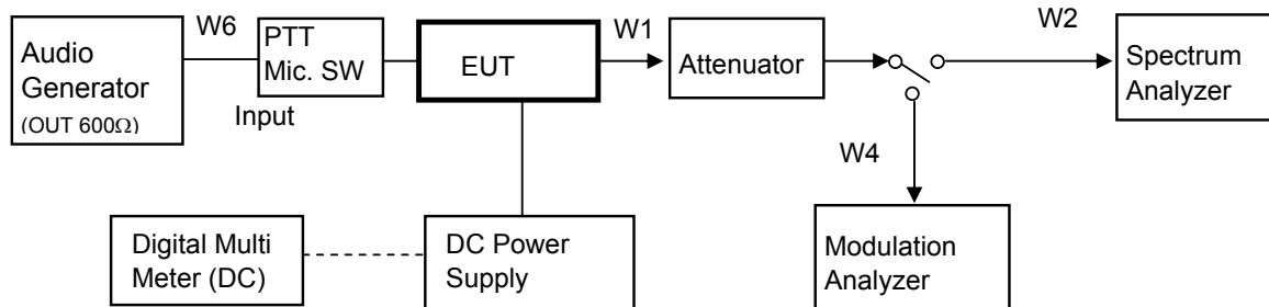
Note: Configuration of other Modulation(4Level FSK) test is composed without the Audio Generator.
