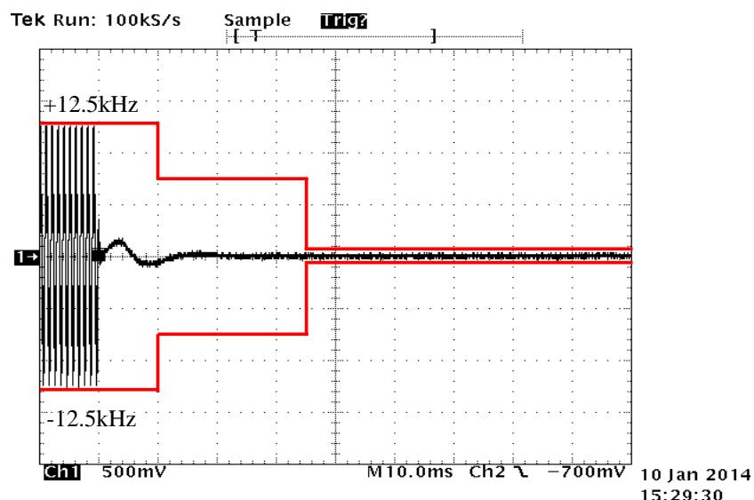
State : High Power / Authorized Bandwidth 11.25 kHz / 11K0F3E / 481.05 MHz / PTT:ON -OFF
