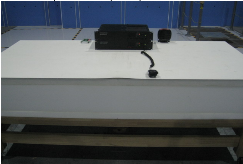
10.10 Receiver Spurious Emission (Radiated) : Front view
