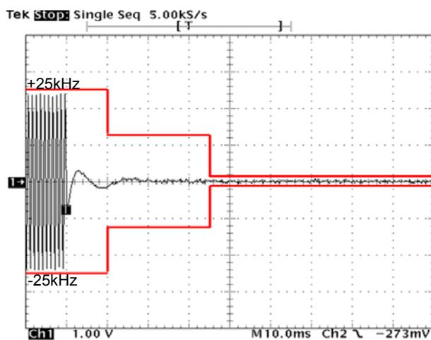
State : High Power / Authorized Bandwidth 20 kHz / 16K0F3E / 469.95 MHz (RSS)/ PTT:ON -OFF
