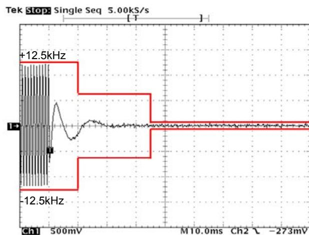
State : High Power / Authorized Bandwidth 11.25 kHz / 7K60FXD/FXE / 429.95 MHz (RSS)/ PTT:ON-OFF
