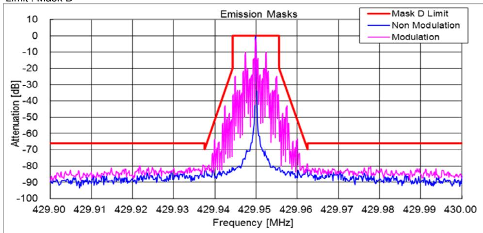
State : High Power / Authorized Bandwidth 11.25 kHz/ 7K60FXD/FXE / 406.15 MHz(FCC)
