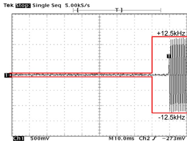
State : High Power / Authorized Bandwidth 11.25 kHz / 7K60FXD/FXE / 429.95 MHz (RSS)/ PTT:OFF -ON
