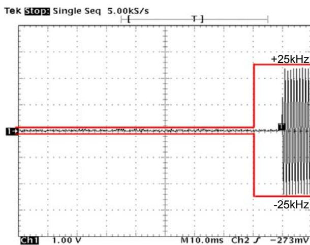
State : High Power / Authorized Bandwidth 11.25 kHz / 11K0F3E / 469.95 MHz (FCC/RSS)/ PTT:OFF -ON
