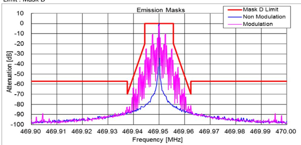
State : Low Power / Authorized Bandwidth 11.25 kHz/ 7K60FXD/FXE / 469.95 MHz(FCC)
