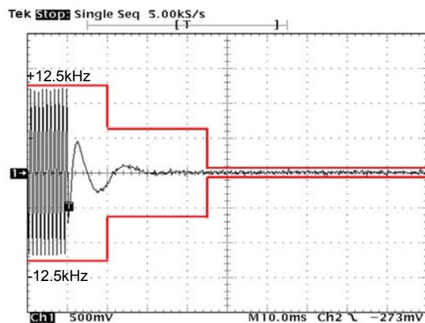
State : High Power / Authorized Bandwidth 11.25 kHz / 11K0F3E / 469.95 MHz (FCC/RSS)/ PTT:ON-OFF
