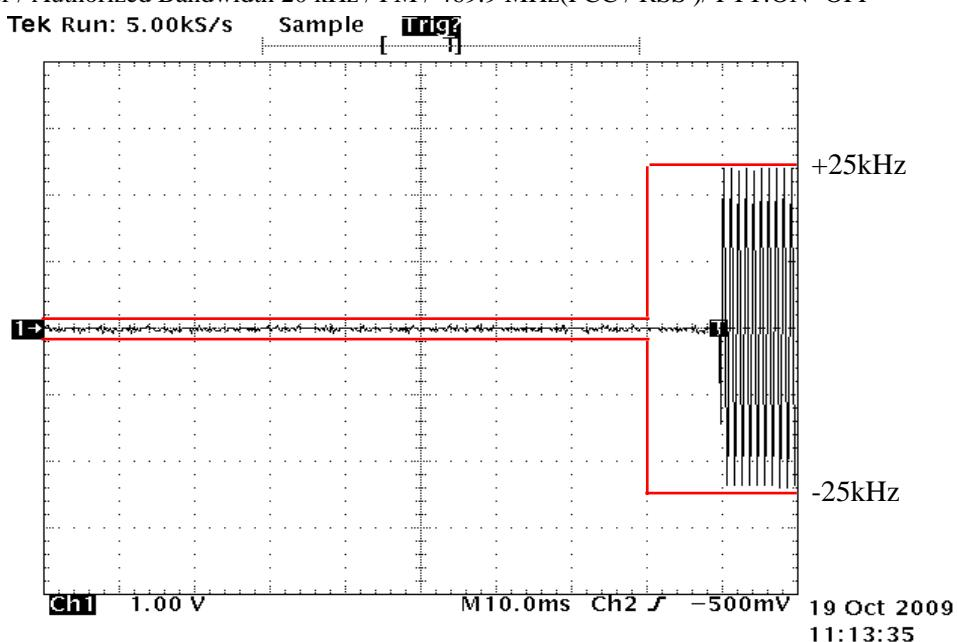
State : High Power / Authorized Bandwidth 11.25 kHz / FM / 469.9 MHz(FCC / RSS ) / PTT:OFF -ON
