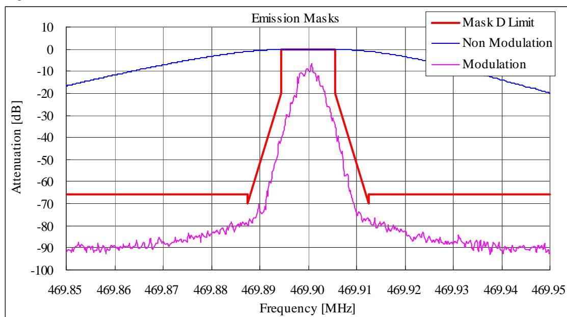
State : High Power / Authorized Bandwidth 6 kHz:4Level FSK / 469.9 MHz(FCC/RSS)
