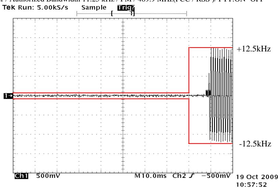
State : High Power / Authorized Bandwidth 11.25 kHz / 4 Lvel FSK / 469.9 MHz(FCC / RSS ) / PTT:OFF -ON
