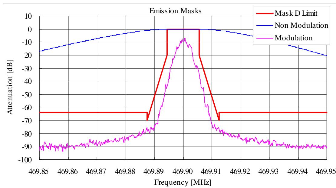
State : Low Power / Authorized Bandwidth 6 kHz:4Level FSK / 469.9 MHz(FCC/RSS)
