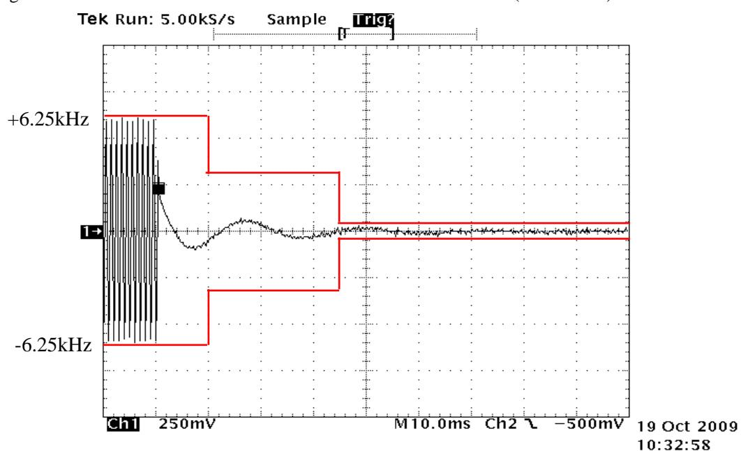
State : High Power / Authorized Bandwidth 6 kHz / 4 Lvel FSK / 469.9 MHz(FCC / RSS )/ PTT:ON -OFF
