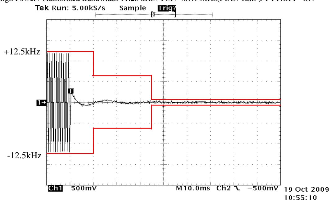
State : High Power / Authorized Bandwidth 11.25 kHz / FM / 469.9 MHz(FCC / RSS ) / PTT:ON -OFF
