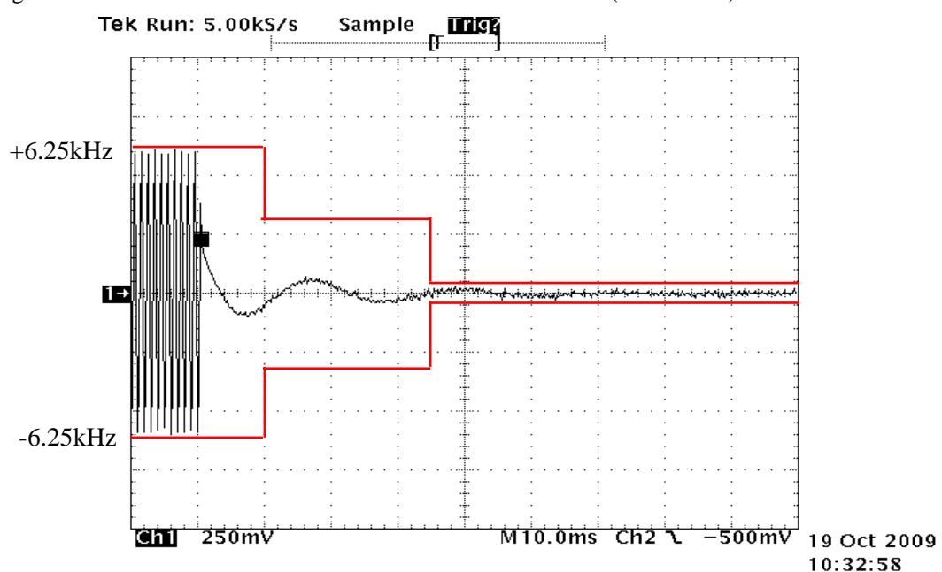
State : High Power / Authorized Bandwidth 6 kHz / CW ID / 469.9 MHz(FCC / RSS )/ PTT:ON -OFF
