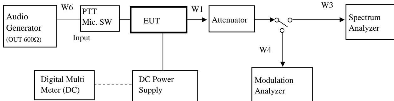
Note: Configuration of other Modulation(4Level FSK) test is composed without the Audio Generator.
