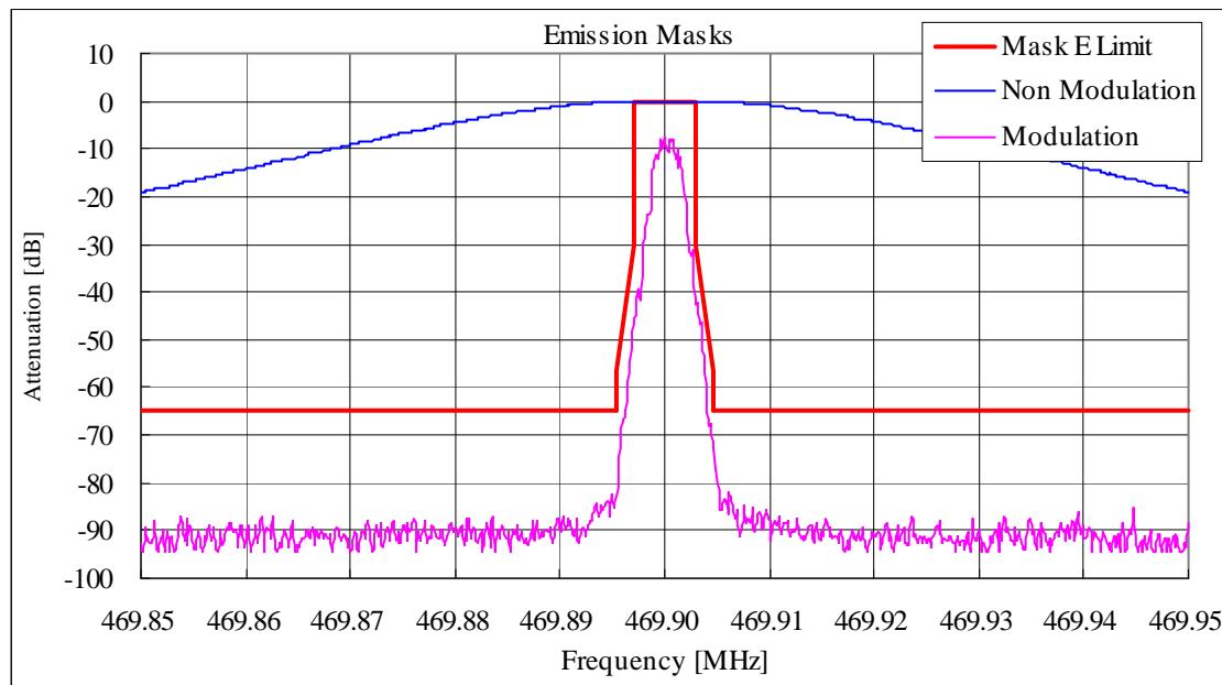
State : Low Power / Authorized Bandwidth 6 kHz:CW ID / 469.9 MHz(FCC)
