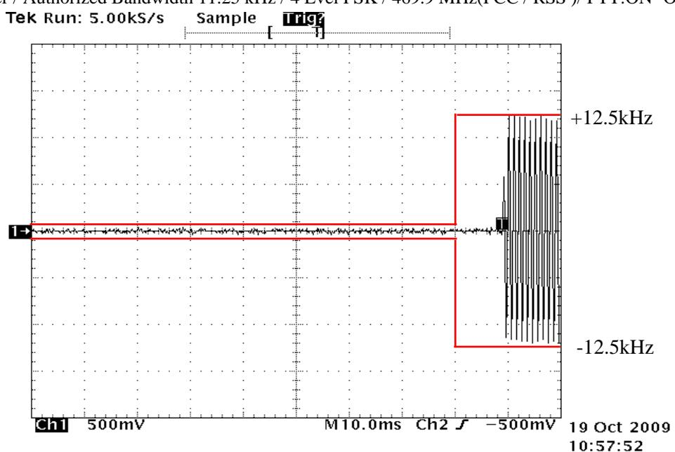
State : High Power / Authorized Bandwidth 6 kHz / 4 Lvel FSK / 469.9 MHz(FCC / RSS )/ PTT:OFF -ON
