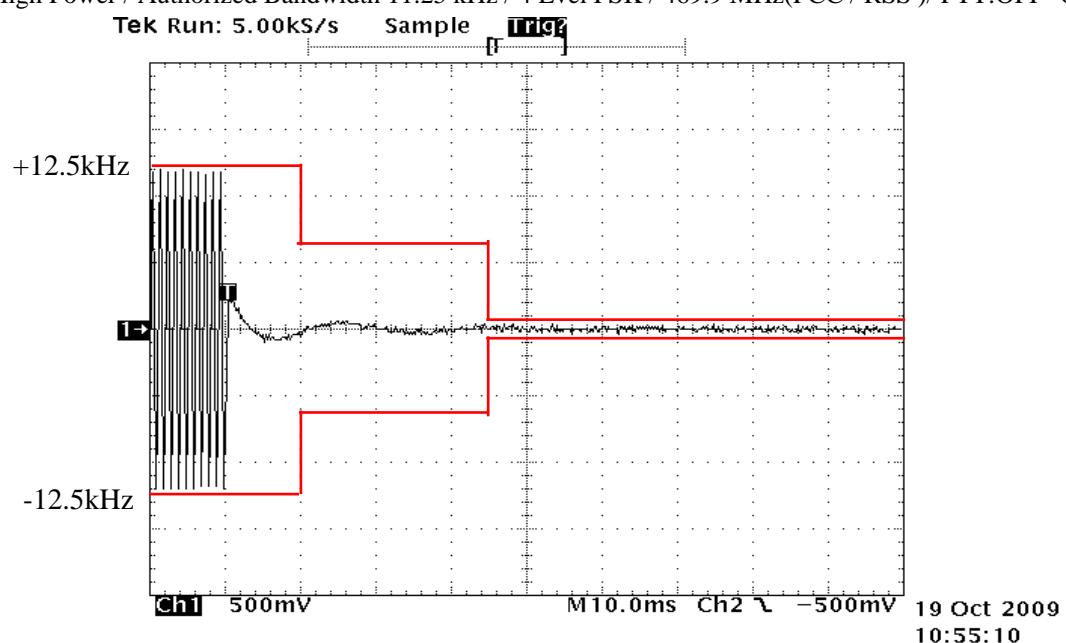
State : High Power / Authorized Bandwidth 11.25 kHz / 4 Lvel FSK / 469.9 MHz(FCC / RSS ) / PTT:ON -OFF
