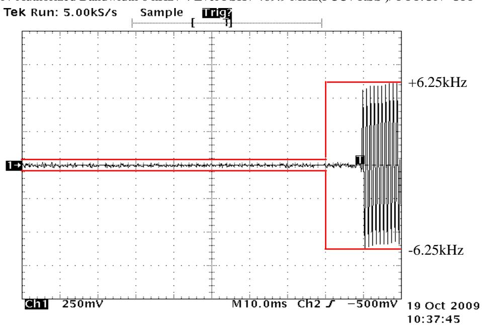
State : High Power / Authorized Bandwidth 6 kHz / CW ID / 469.9 MHz(FCC / RSS )/ PTT:OFF -ON
