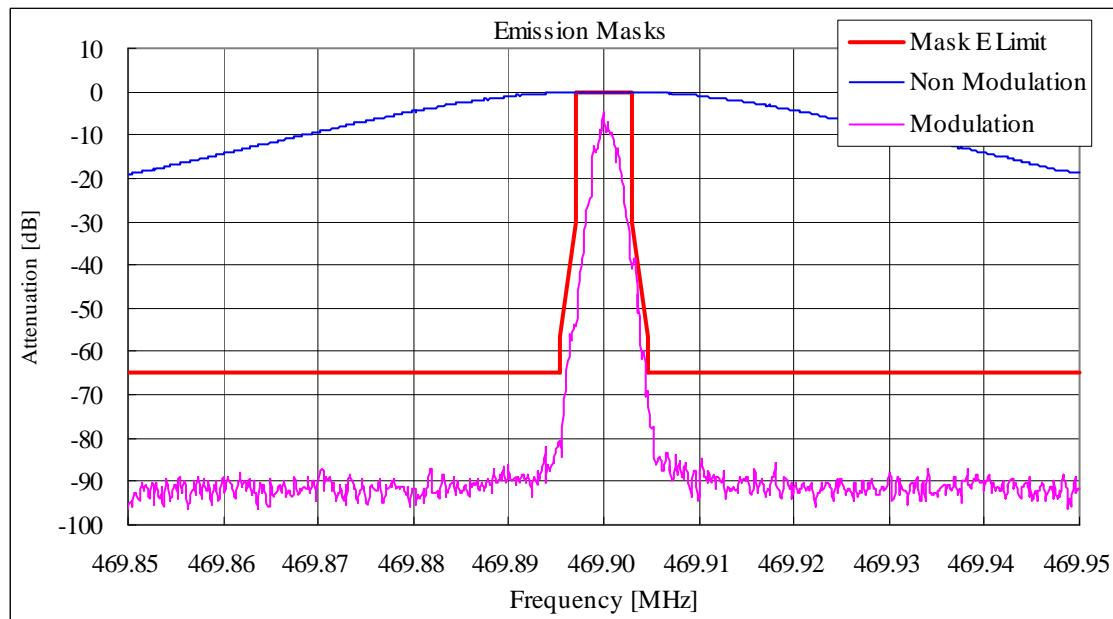
State : High Power / Authorized Bandwidth 6 kHz: CW ID / 469.9 MHz(FCC)
