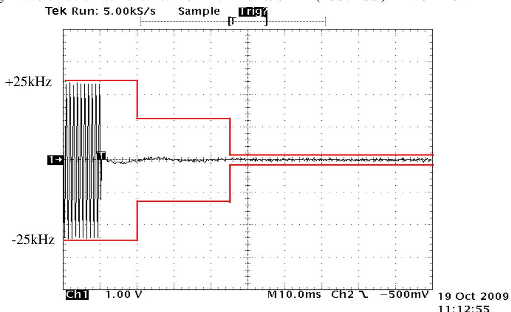
State : High Power / Authorized Bandwidth 20 kHz / FM / 469.9 MHz(FCC / RSS ) / PTT:ON -OFF
