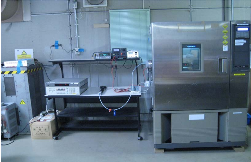
10.8, 10.9 Frequency Stability : Outer view
