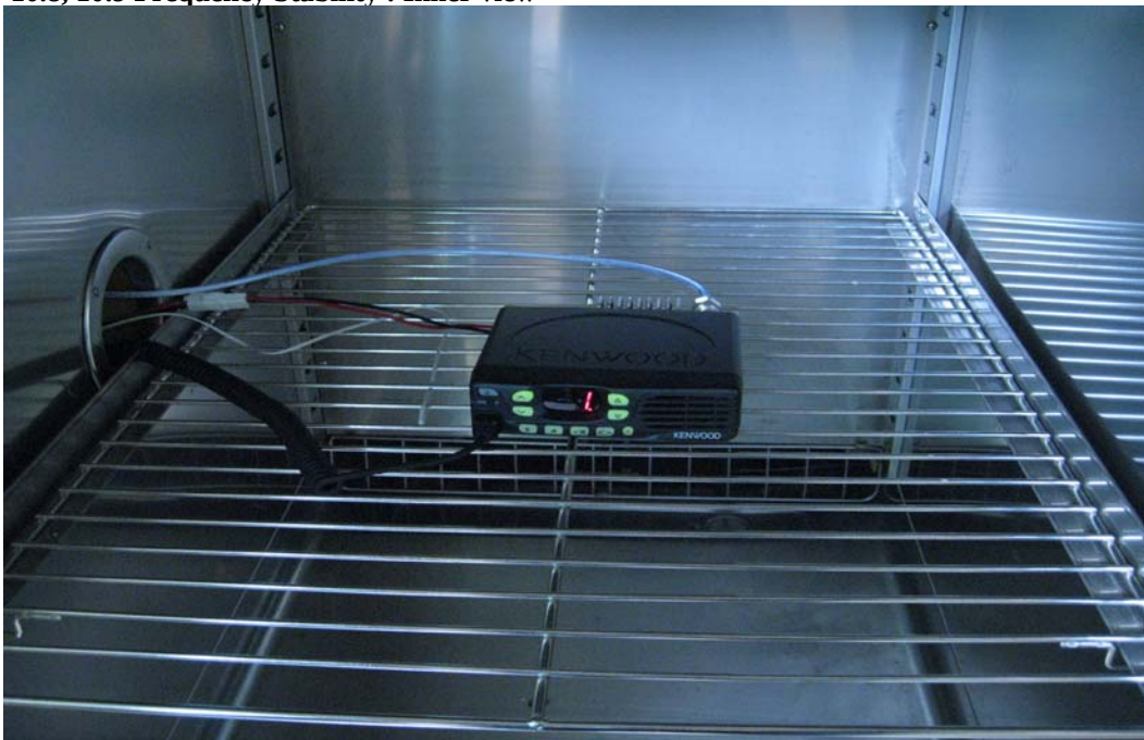
10.8, 10.9 Frequency Stability : Inner view
