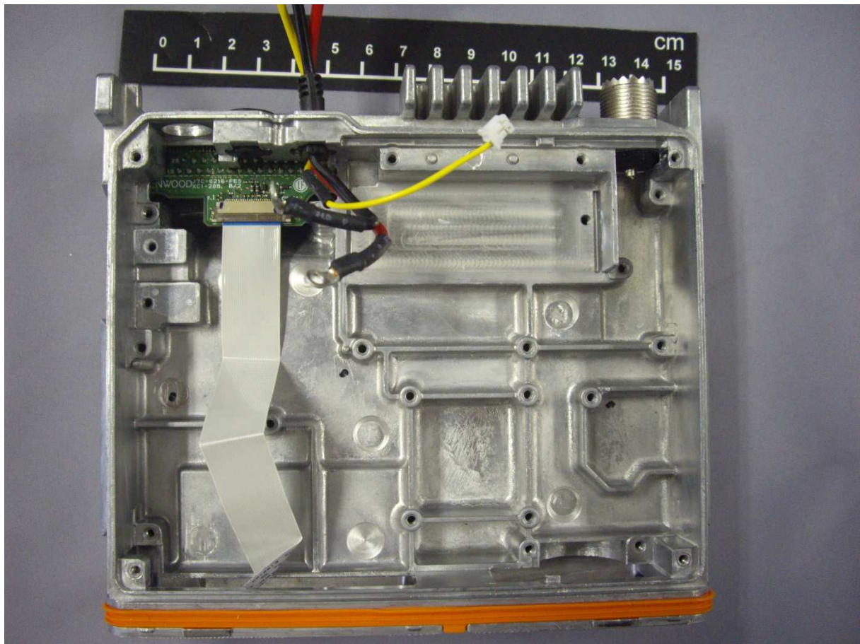
Internal View of D-Sub Unit
