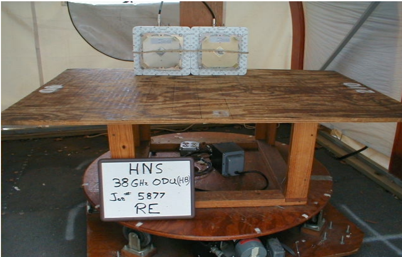
Figure 36 Test setup photo 1 for Open field Site for Radiated Spurious Emission for Both Hub and Sub 38 GHz High band ODUS (30Mhz- 18 GHz)
